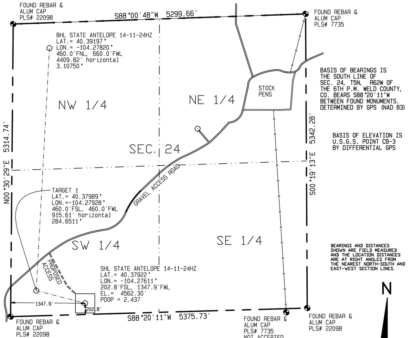
I HEREBY CERTIFY THAT THIS PLAT IS AN ACCURATE REPRESENTATION OF A CORRECT SURVEY SHOWING THE LOCATION OF SAID WELLSITE:
