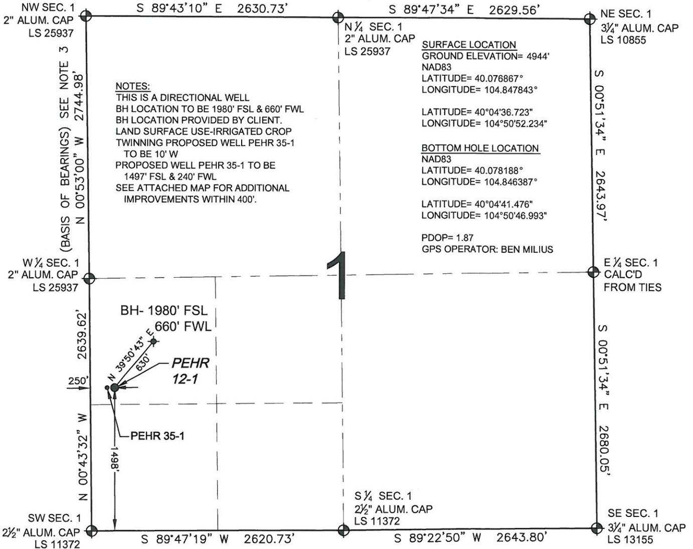
WELL PEHR 12-1 TO BE LOCATED 1498' FSL AND 250' FWL, SECTION 1, T1N, R67W OF THE 6th P.M.
