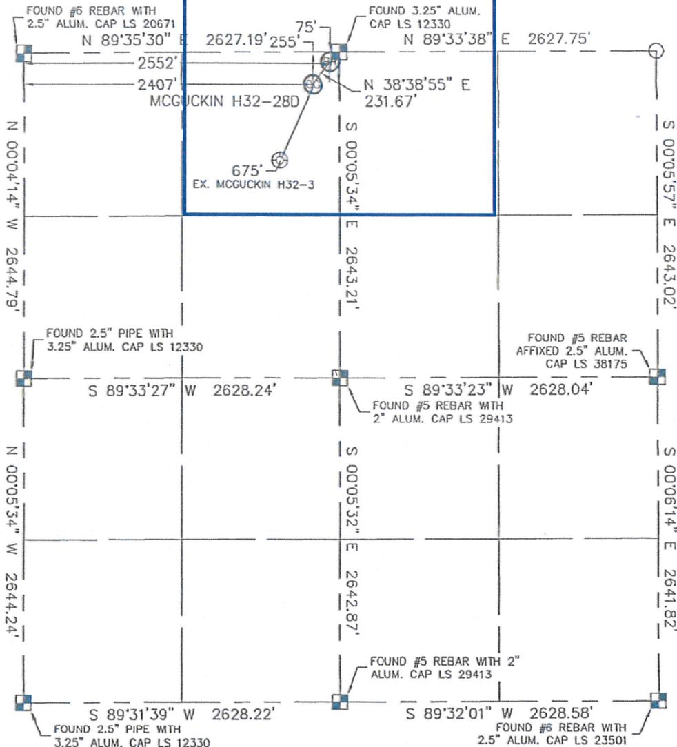
In accordance with a request from Erik Van Decar with Noble Energy Inc. Lat40°, Inc. has determined the surface location of the MCGUCKIN H32-28D to be 255' from the NORTH line and 2407' from the WEST line and the bottom hole to be 75' from the NORTH line and 2552' from the WEST line as measured at right angles from the section lines of Section 32, Township 3 North, Range 65 West of the Sixth Principal Meridian, County of Weld, State of Colorado.
