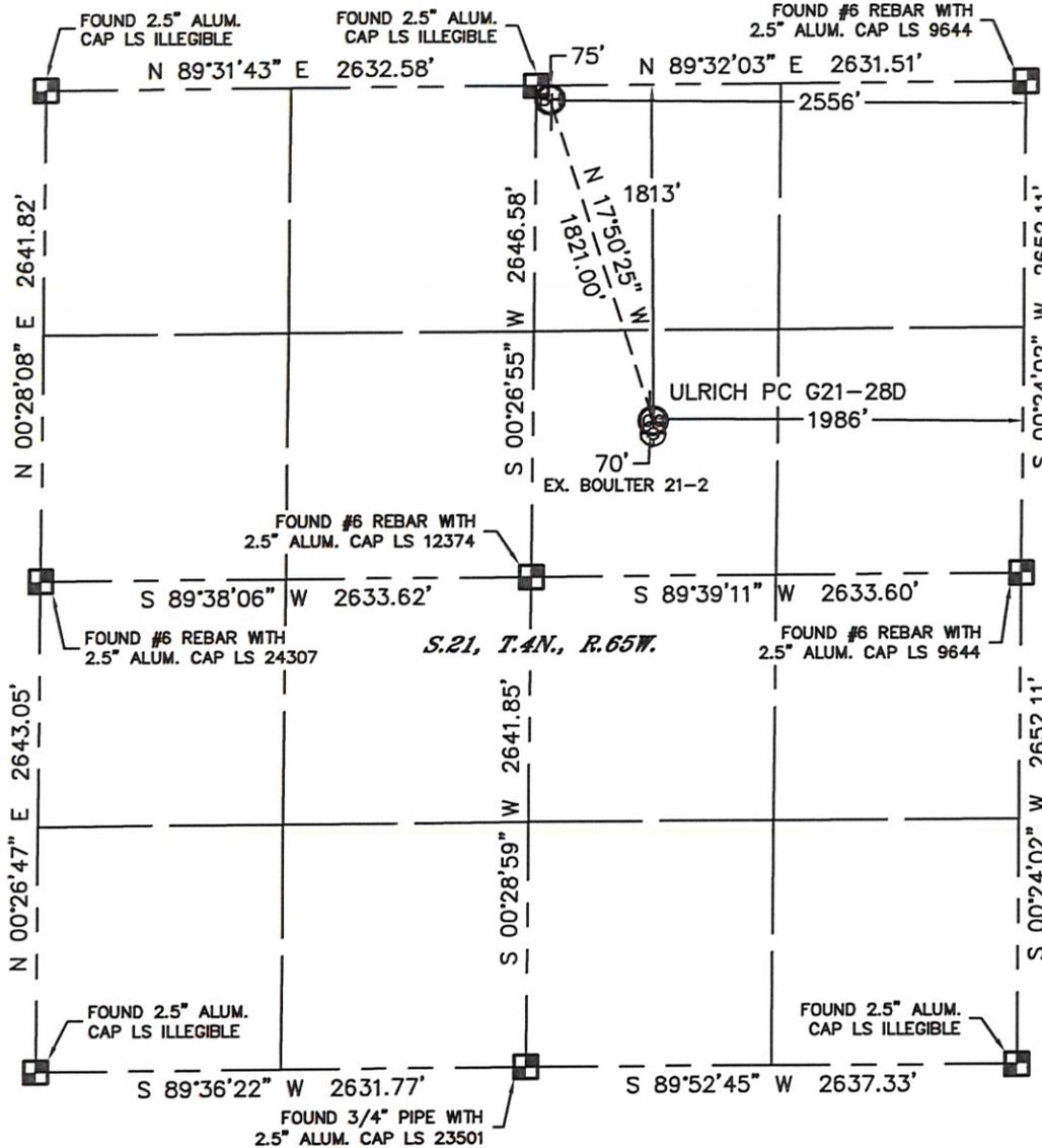
In accordance with a request from Ryan Hawkins with Noble Energy Inc. Lat40°, Inc. has determined the surface location of the ULRICH PC G21-28D to be 1813' from the NORTH line and 1986' from the EAST line and the bottom hole to be 75' from the NORTH line and 2556' from the EAST line as measured at right angles from the section lines of Section 21, Township 4 North, Range 65 West of the Sixth Principal Meridian, County of Weld, State of Colorado.
