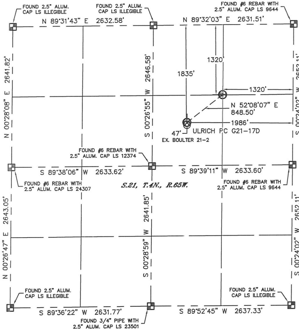
In accordance with a request from Ryan Hawkins with Noble Energy Inc. Lat40°, Inc. has determined the surface location of the ULRICH PC G21-17D to be 1835' from the NORTH line and 1986' from the EAST line and the bottom hole to be 1320' from the NORTH line and 1320' from the EAST line as measured at right angles from the section lines of Section 21, Township 4 North, Range 65 West of the Sixth Principal Meridian, County of Weld, State of Colorado.
