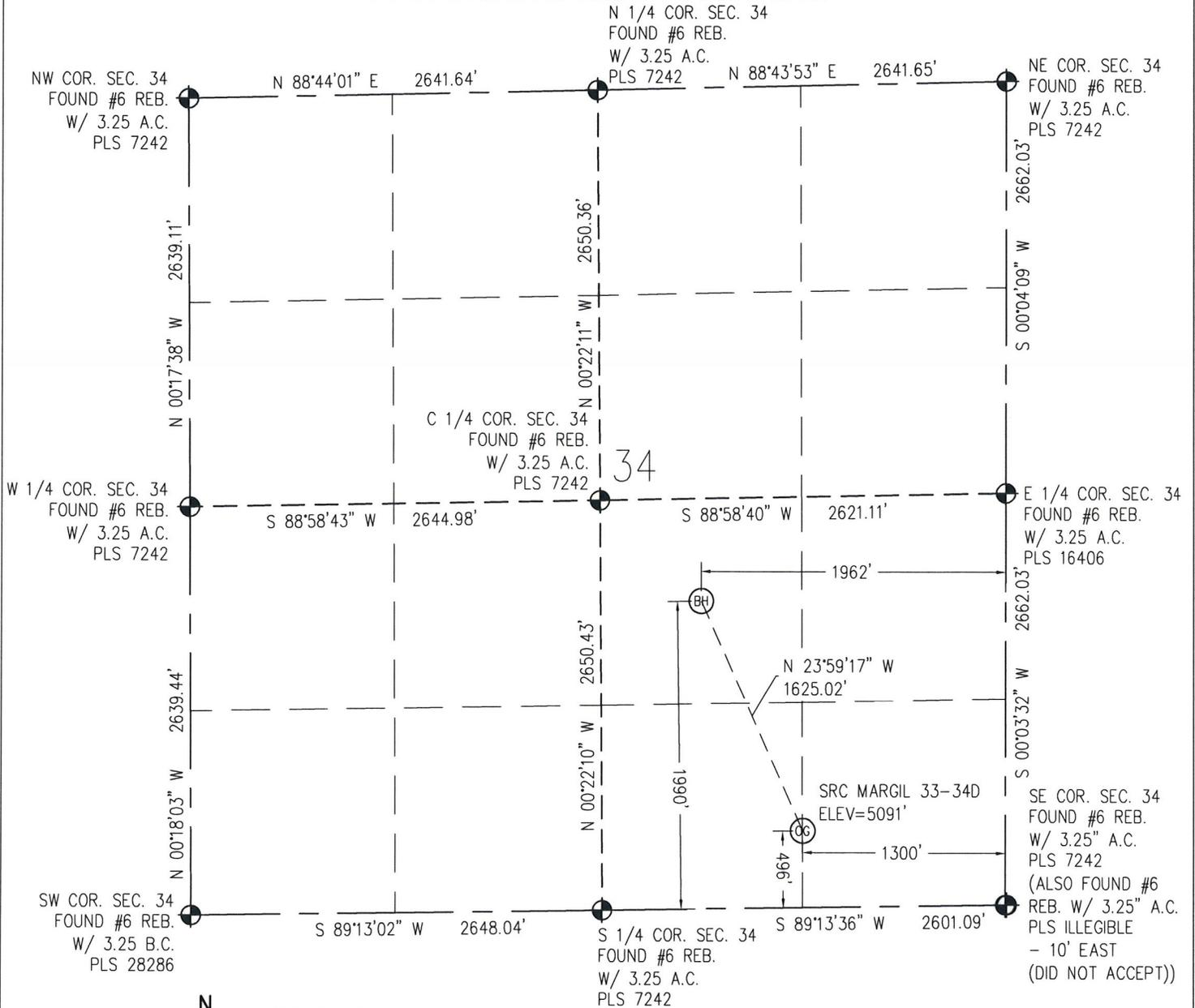
IN ACCORDANCE WITH A REQUEST FROM CRAIG RASMUSON - SYNERGY RESOURCES, BASELINE ENGINEERING CORP. HAS DETERMINED THE LOCATION OF THE SRC MARGIL 33-34D TO BE 496' FSL AND 1,300' FEL, AS MEASURED AT NINETY (90) DEGREES FROM THE SECTION LINE OF SECTION 34, TOWNSHIP 4 NORTH, RANGE 68 WEST AND THE BOTTOM HOLE LOCATION TO BE 1,990' FSL AND 1,962' FEL OF SECTION 34, TOWNSHIP 4 NORTH, RANGE 68 WEST, 6TH PRINCIPAL MERIDIAN, WELD COUNTY, COLORADO.
