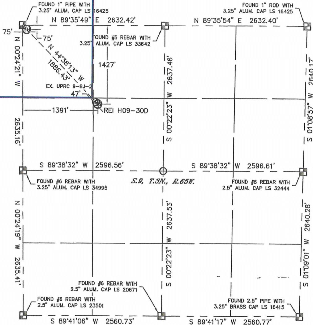
In accordance with a request from Iony Patterson with Noble Energy Inc., Lat40°, Inc. has determined the surface location of the REI H09-300 to be 1427' from the NORTH line and 1391' from the WEST line and the bottom hole to be 75' from the NORTH line and 75' from the WEST line as measured at right angles from the section lines of Section 9, Township 3 North, Range 65 West of the Sixth Principal Meridian, County of Weld, State of Colorado.
