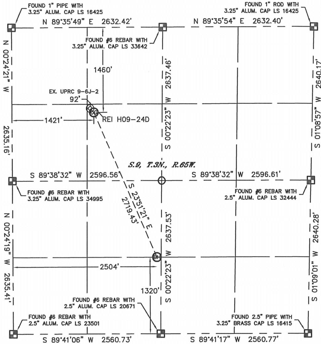
In accordance with a request from Tony Patterson with Noble Energy Inc. Lat40°, Inc. has determined the surface location of the REI H09-24D to be 1460' from the NORTH line and 1421' from the WEST line and the bottom hole to be 1320' from the SOUTH line and 2504' from the WEST line as measured at right angles from the section lines of Section 9, Township 3 North, Range 65 West of the Sixth Principal Meridian, County of Weld, State of Colorado.
