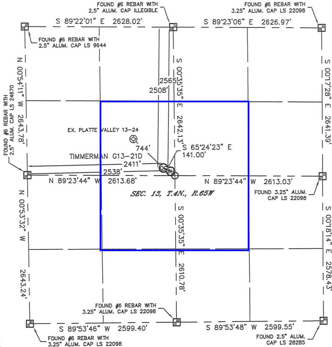
In accordance with a request from Nate McCorkell with Noble Energy Inc. Lat40°, Inc. has determined the surface location of the Timmerman G13-21D to be 2508' from the NORTH line and 2411' from the WEST line and the bottom hole to be 2565' from the NORTH line and 2538' from the WEST line as measured at right angles from the section lines of Section 13, Township 4 North, Range 65 West of the Sixth Principal Meridian, County of Weld, State of Colorado.
