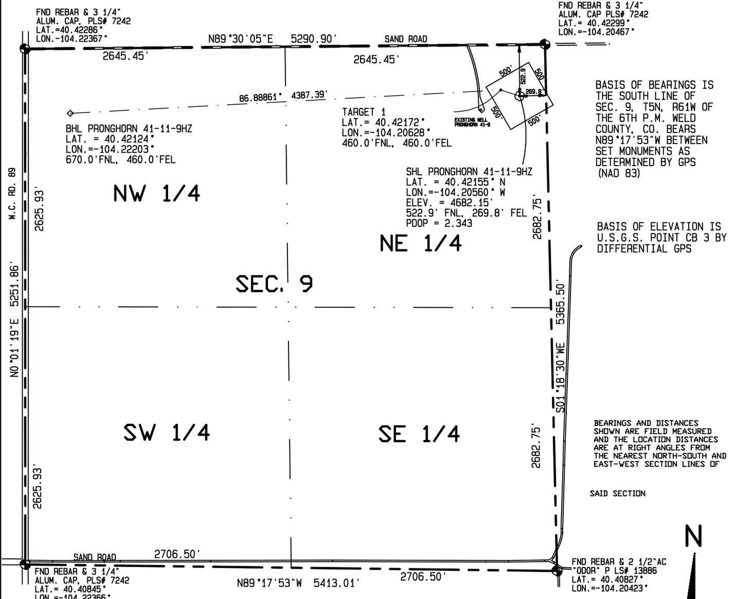
BASIS OF BEARINGS IS THE SOUTH LINE OF SEC. 9, T5N, R61W OF THE 6TH P.M. WELD COUNTY, CO. BEARS N89°17'53\"W BETWEEN SET MONUMENTS AS DETERMINED BY GPS (NAD 83)
