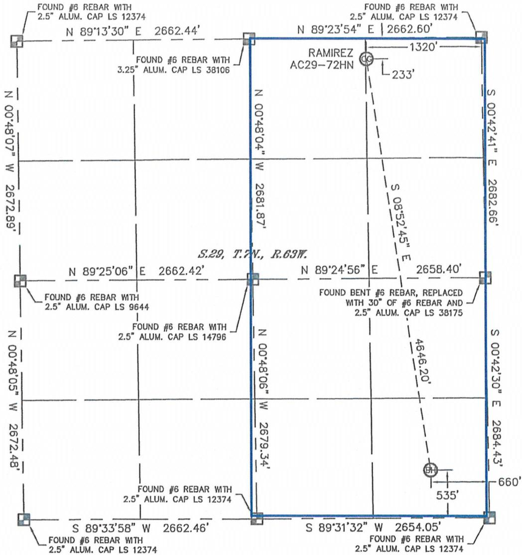
In accordance with a request from Jacob Rice with Noble Energy Inc. Lat40°, Inc. has determined the surface location of the RAMIREZ AC29-72HN to be 233' from the NORTH line and 1320' from the EAST line and the bottom hole to be 535' from the SOUTH line and 660' from the EAST line as measured at right angles from the section lines of Section 29, Township 7 North, Range 63 West of the Sixth Principal Meridian, County of Weld, State of Colorado.
