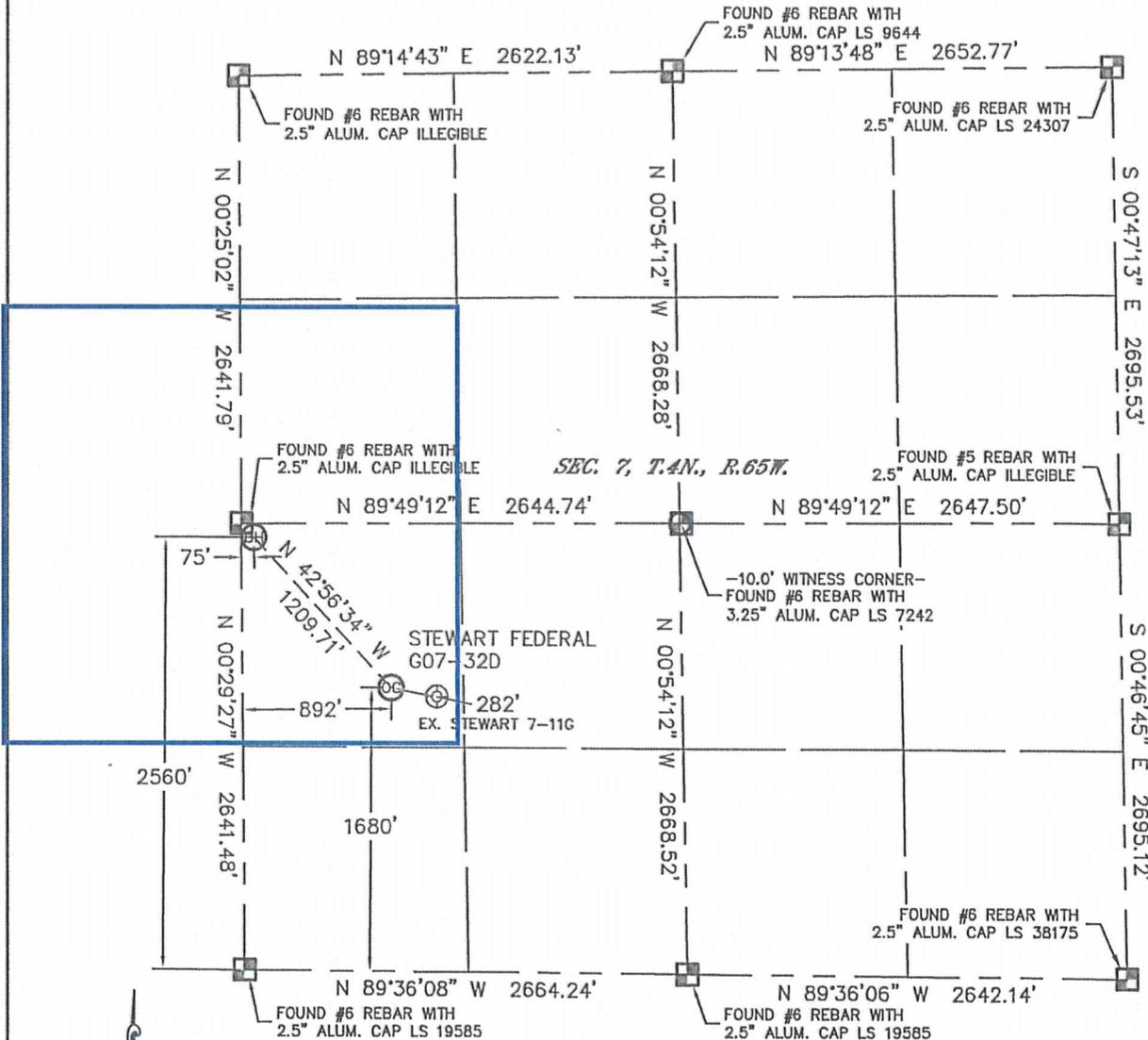
In accordance with a request from Matt Verbit with Noble Energy Inc., Lat40°, Inc. has determined the surface location of the STEWART FEDERAL G07-32D to be 1680' from the SOUTH line and 892' from the WEST line and the bottom hole to be 2560' from the SOUTH line and 75' from the WEST line as measured at right angles from the section lines of Section 7, Township 4 North, Range 65 West of the Sixth Principal Meridian, County of Weld, State of Colorado.
