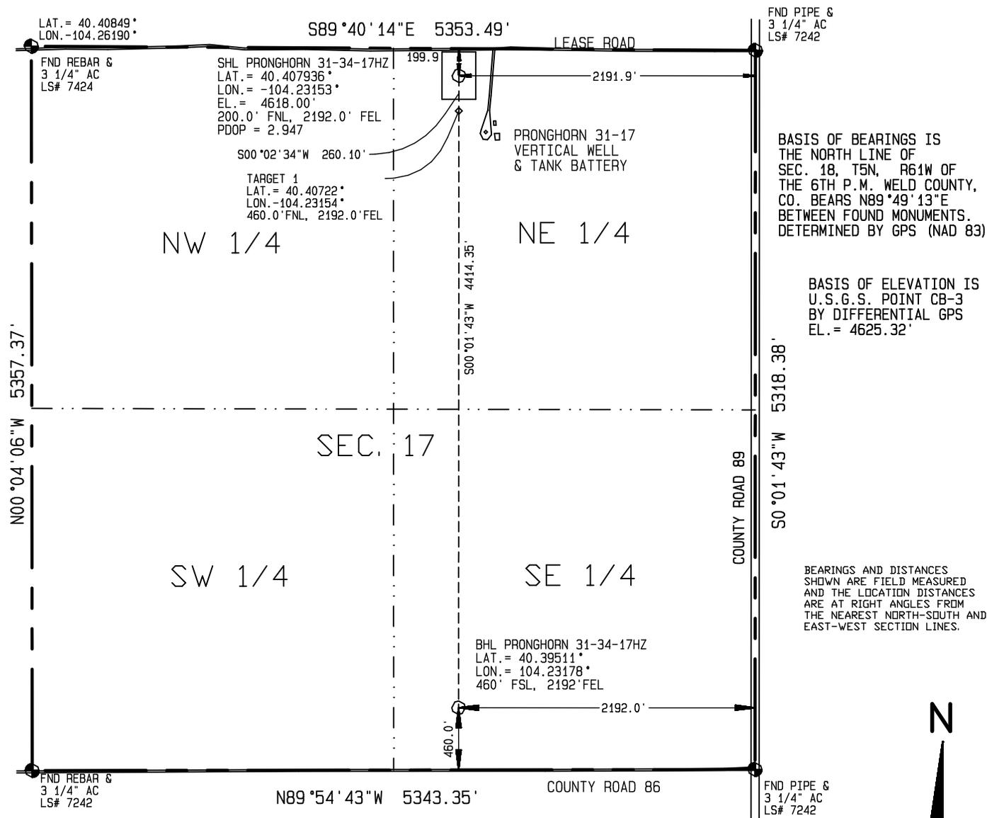
BASIS OF BEARINGS IS THE NORTH LINE OF SEC. 18, T5N, R61W OF THE 6TH P.M. WELD COUNTY, CO. BEARS N89°49'13"E BETWEEN FOUND MONUMENTS. DETERMINED BY GPS (NAD 83)
