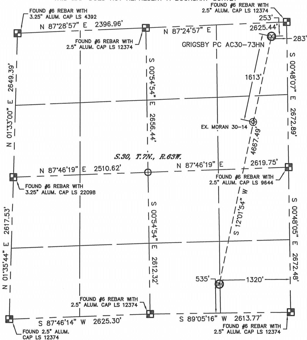
In accordance with a request from Jacob Rice with Noble Energy Inc. Lat40°, Inc. has determined the surface location of the GRIGSBY PC AC30-73HN to be 253' from the NORTH line and 283' from the EAST line and the bottom hole to be 535' from the SOUTH line and 1320' from the EAST line as measured at right angles from the section lines of Section 30, Township 7 North, Range 63 West of the Sixth Principal Meridian, County of Weld, State of Colorado.
