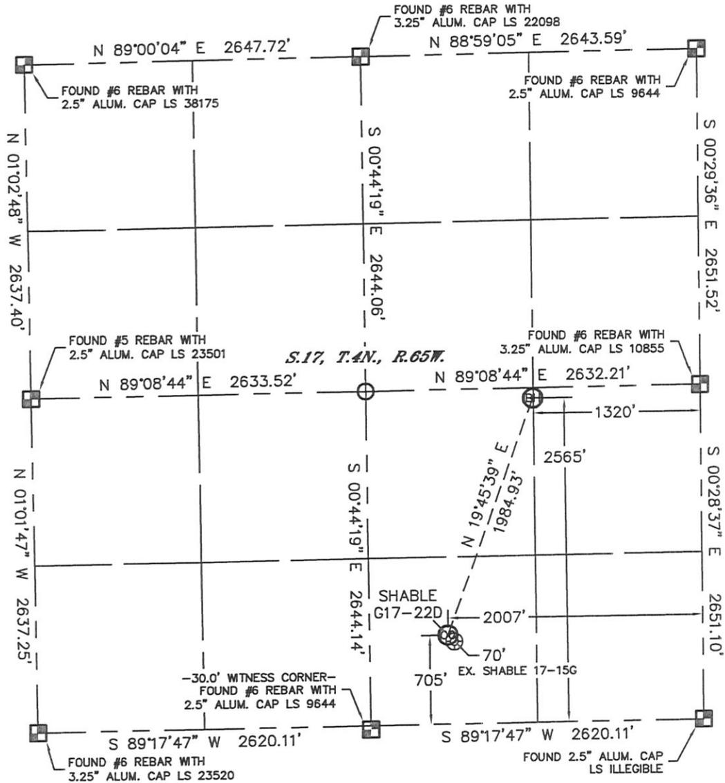
In accordance with a request from Ryan Hawkins with Noble Energy Inc. Lat40°, Inc. has determined the surface location of the SHABLE G17-22D to be 705' from the SOUTH line and 2007' from the EAST line and the bottom hole to be 2565' from the SOUTH line and 1320' from the EAST line as measured at right angles from the section lines of Section 17, Township 4 North, Range 65 West of the Sixth Principal Meridian, County of Weld, State of Colorado.
