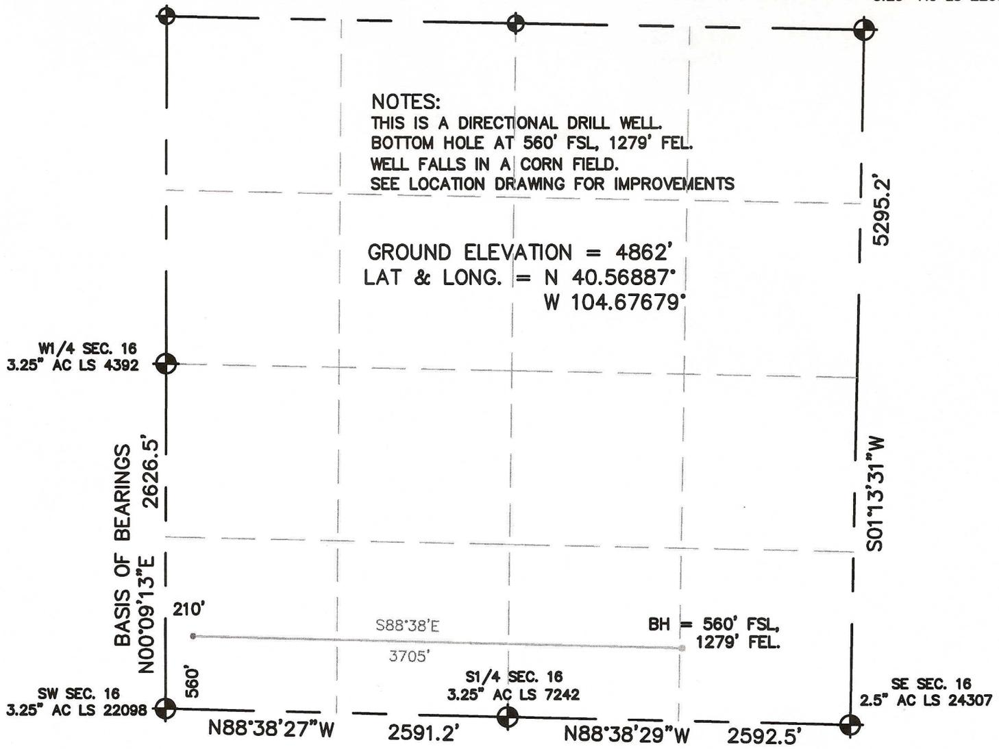
I HEREBY STATE TO PETROLEUM DEV. CORP. THAT THIS WELL LOCATION CERTIFICATE FOR THE WELL MOSS 14-16H IS LOCATED 560' FSL & 210' FWL, SEC. 16, T7N, R65W, 6PM.
