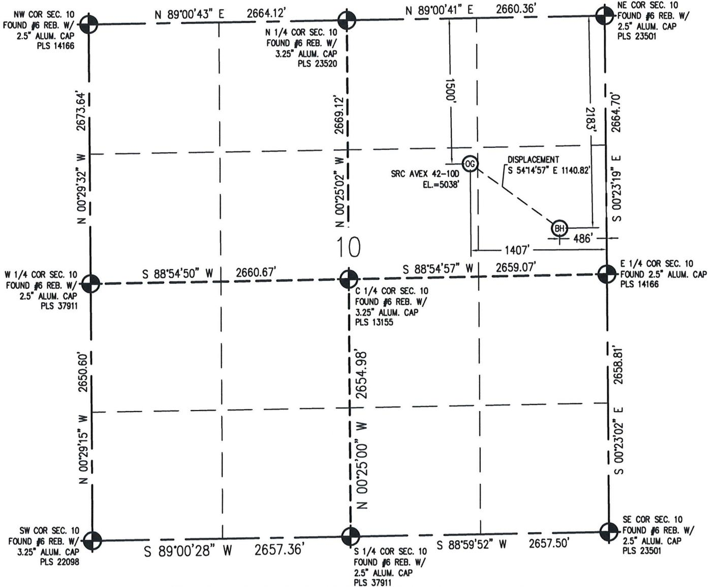
IN ACCORDANCE WITH A REQUEST FROM CRAIG RASMUSON - SYNERGY RESOURCES, BASELINE ENGINEERING CORP. HAS DETERMINED THE LOCATION OF THE SRC AVEX 42-10D TO BE 1500' FNL, 1407' FEL, AS MEASURED AT NINETY (90) DEGREES FROM THE SECTION LINE OF SECTION 10, TOWNSHIP 4 NORTH, RANGE 68 WEST AND THE BOTTOM HOLE LOCATION TO BE 2183' FNL AND 486' FEL OF SECTION 10, TOWNSHIP 4 NORTH, RANGE 68 WEST, 6TH PRINCIPAL MERIDIAN, WELD COUNTY, COLORADO.
