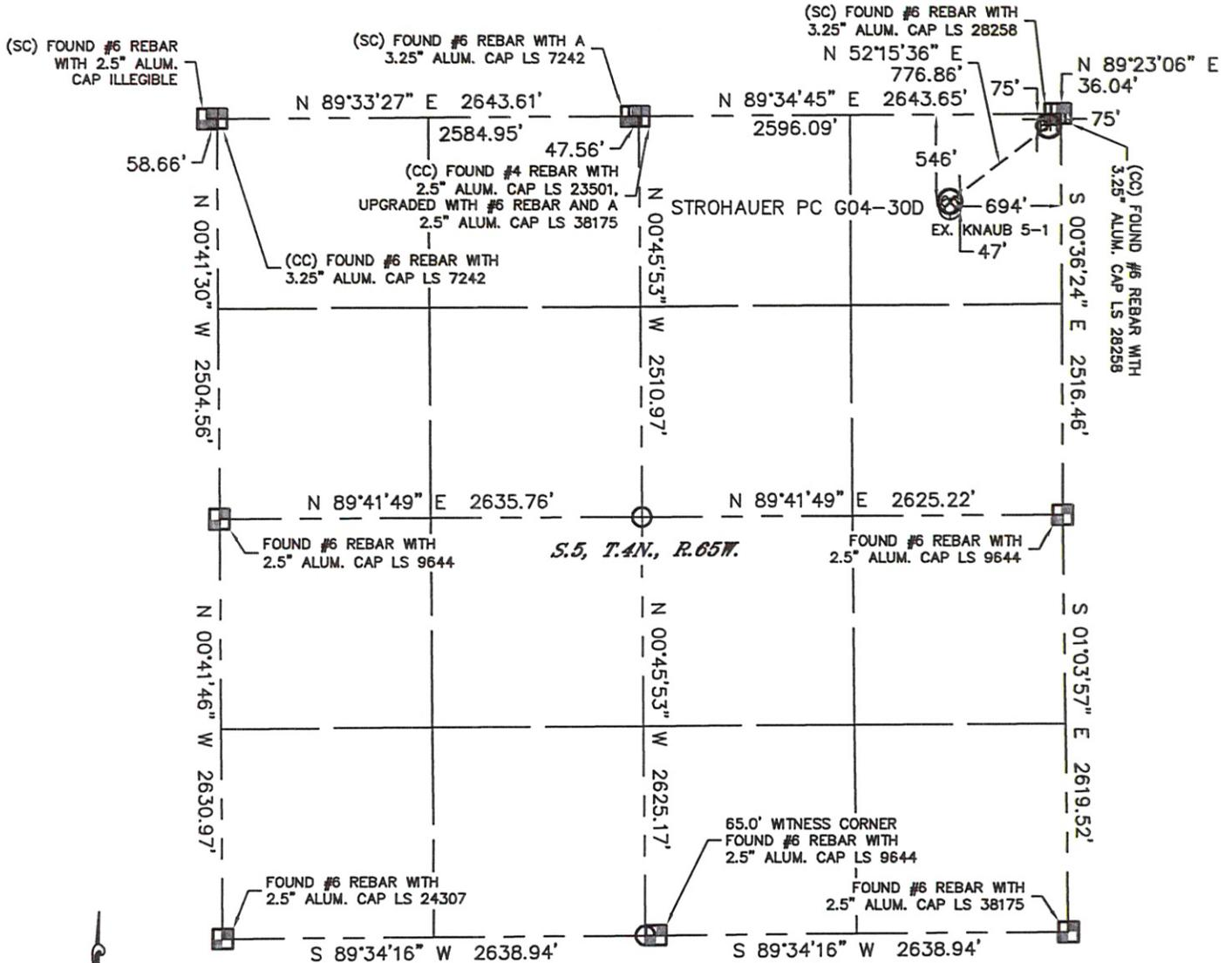
In accordance with a request from Brian DeRose with Noble Energy Inc. Lat40°, Inc. has determined the surface location of the STROHAUER PC G04-30D to be 546' from the NORTH line and 694' from the EAST line and the bottom hole to be 75' from the NORTH line and 75' from the EAST line as measured at right angles from the section lines of Section 5, Township 4 North, Range 65 West of the Sixth Principal Meridian, County of Weld, State of Colorado.
