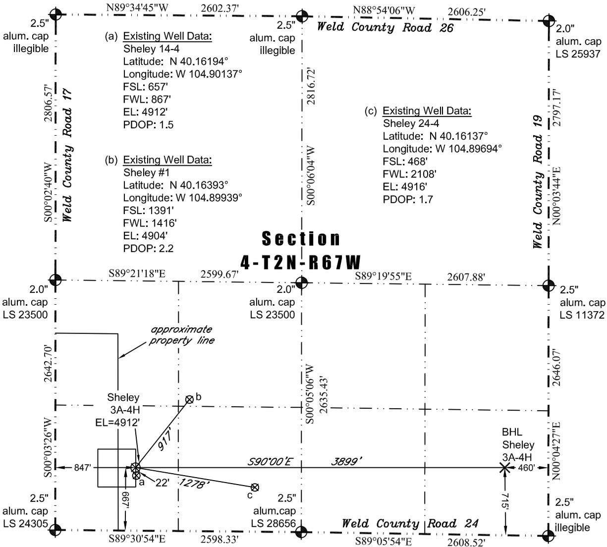
In accordance with a request from Jay Knutson of EnCana Oil & Gas (USA) Inc., PLS Group, LLC has determined the location of the **Sheley 3A-4H** well site to be SHL: 667' FSL and 847' FWL, (BHL 715' FSL and 460' FEL), as measured at ninety (90) degrees from the section lines of Section 4, Township 2 North, Range 67 West of the 6th Principal Meridian, Weld County Colorado.
