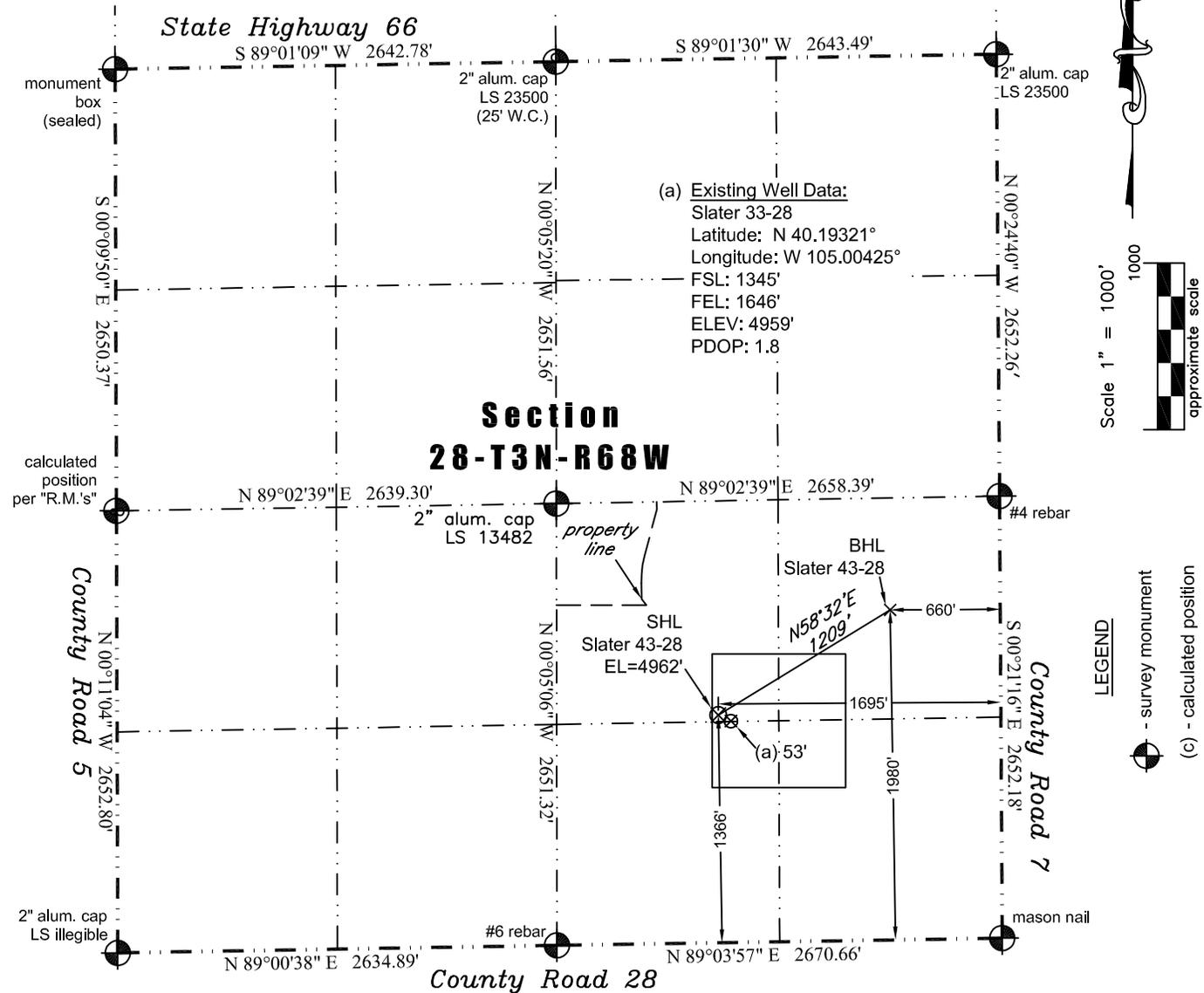
In accordance with a request from Jay Knutson of EnCana Oil & Gas (USA) Inc., PLS Group, LLC has determined the location of the **Slater 43-28** well site to be SHL: 1366' FSL and 1695' FEL, (BHL 1980' FSL and 660' FEL) as measured at ninety (90) degrees from the section lines of Section 28, Township 3 North, Range 68 West, 6th Principal Meridian, County of Weld, CO.
