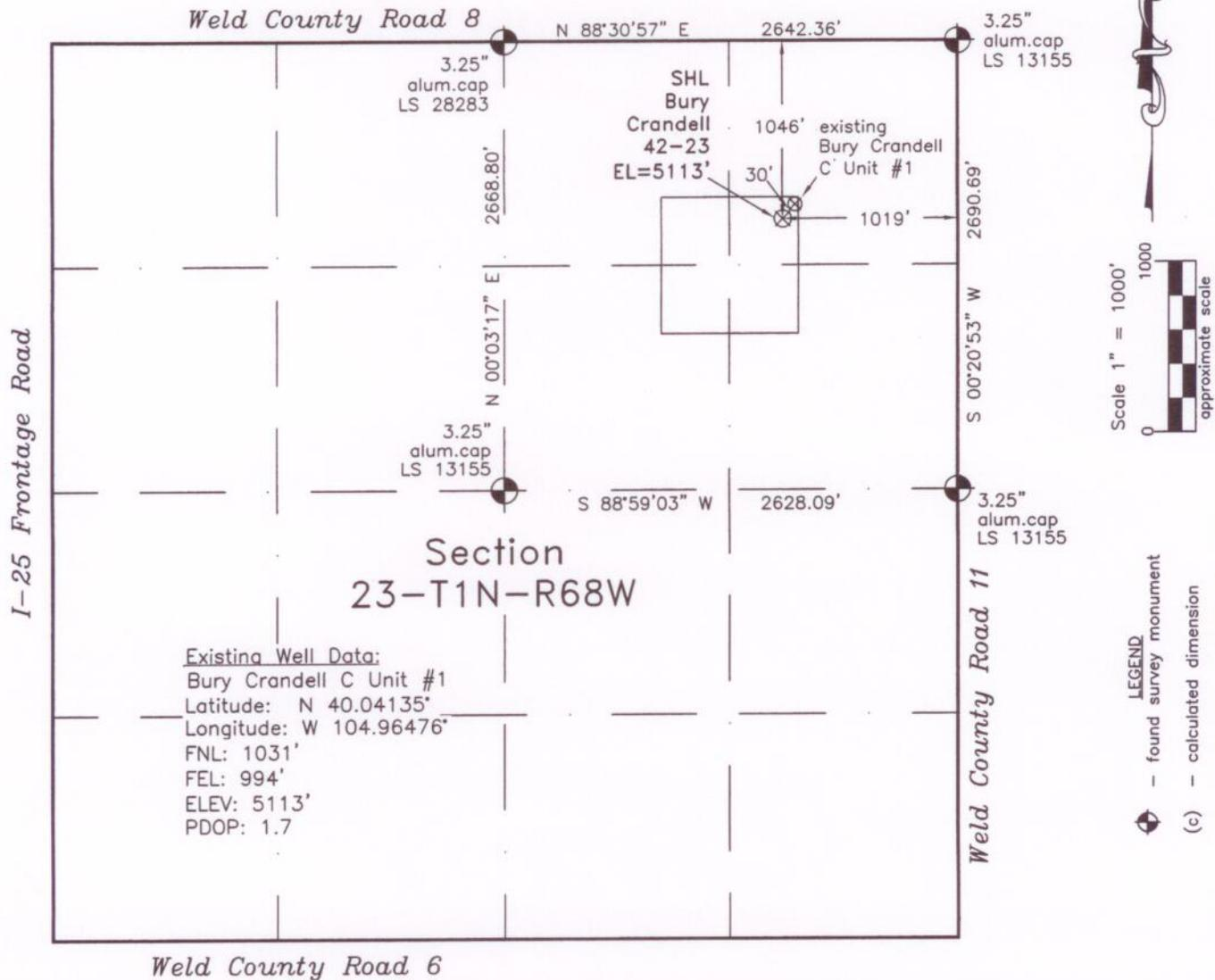
In accordance with a request from Doug Pearlman of EnCana Oil & Gas (USA) Inc., Frederick Land Surveying, Inc. has determined the location of the **Bury Crandell 42-23** well site to be SHL: 1046' FNL and 1019' FEL, as measured at ninety (90) degrees from the section lines of Section 23, Township 1 North, Range 68 West, 6th Principal Meridian, City and County of Broomfield, CO.
