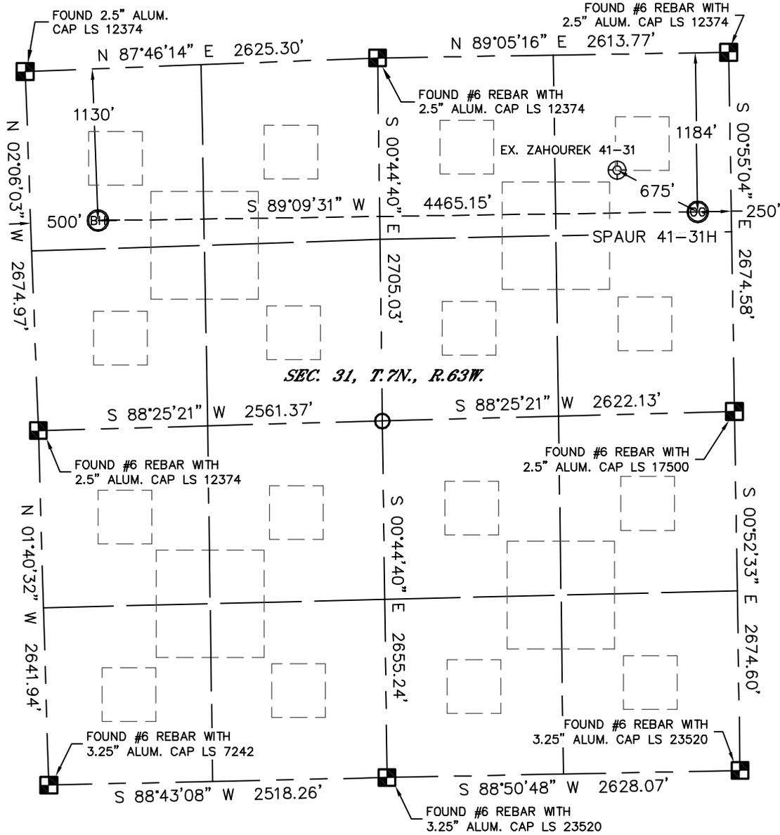
In accordance with a request from Thomas Bragg with PDC Energy Lat40°, Inc. has determined the surface location of the SPAUR 41-31H to be 1184' from the NORTH line and 250' from the EAST line and the bottom hole to be 1130' from the NORTH line and 500' from the WEST line as measured at right angles from the section lines of Section 31, Township 7 North, Range 63 West of the Sixth Principal Meridian, County of Weld, State of Colorado.
