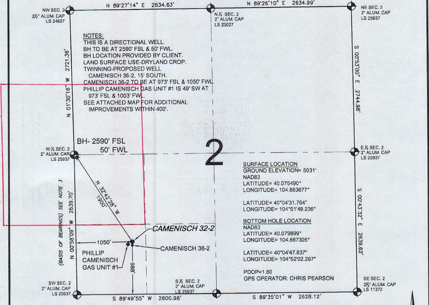
WELL CAMENISCH 32-2 TO BE LOCATED 988' FSL AND 1050' FWL, SECTION 2, T1N, R67W OF THE 6th P.M.
