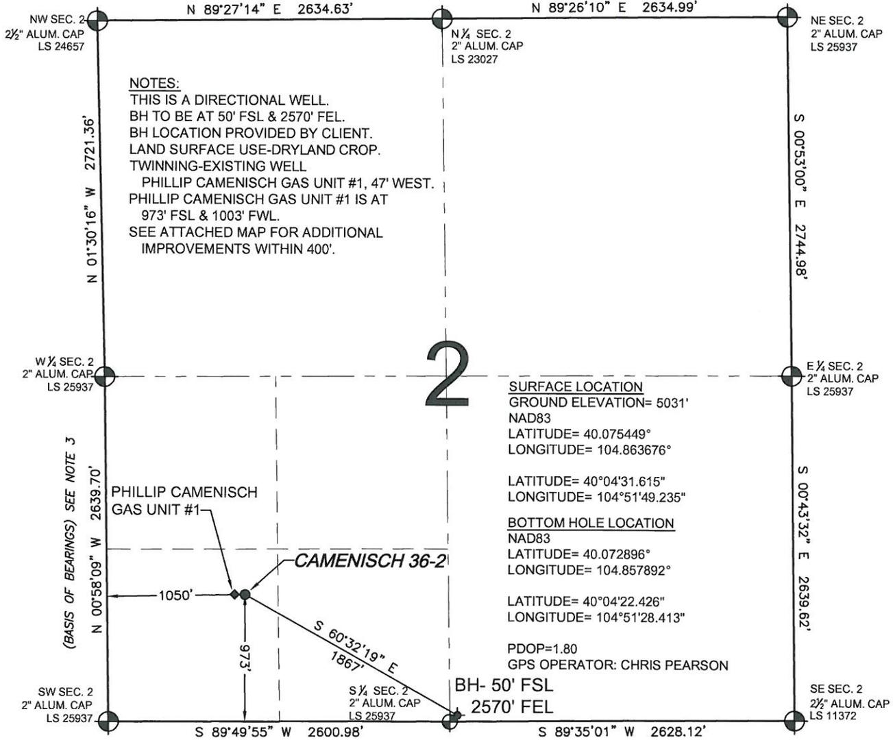
WELL CAMENISCH 36-2 TO BE LOCATED 973' FSL AND 1050' FWL, SECTION 2, T1N, R67W OF THE 6th P.M.
