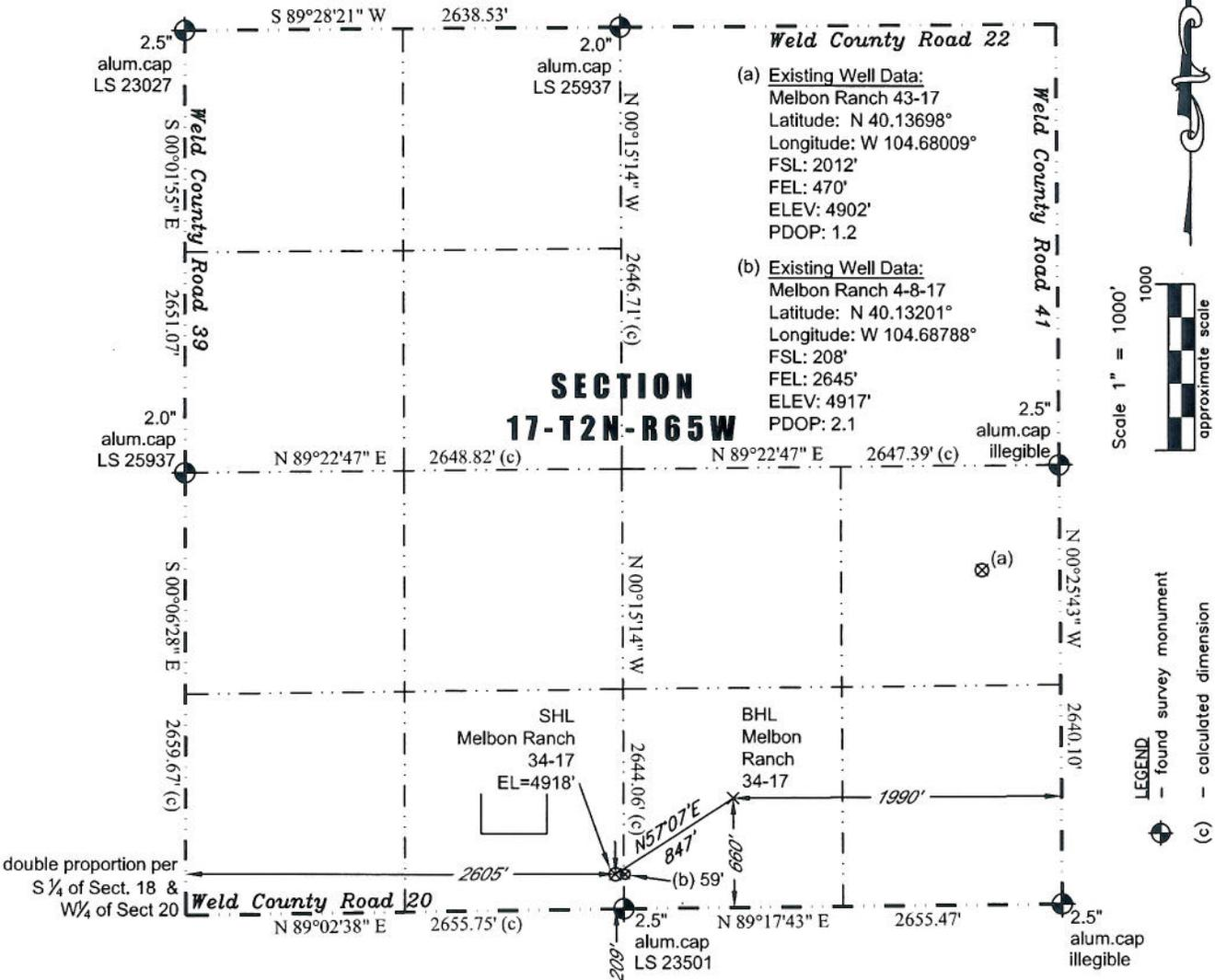
In accordance with a request from Jay Knutson of EnCana Oil & Gas (USA) Inc., PLS Group, LLC has determined the location of the **Melbon Ranch 34-17** well site to be SHL: 209' FSL and 2605' FWL, (BHL 660' FSL and 1990' FEL), as measured at ninety (90) degrees from the section lines of Section 17, Township 2 North, Range 65 West of the 6th Principal Meridian, Weld County Colorado.
