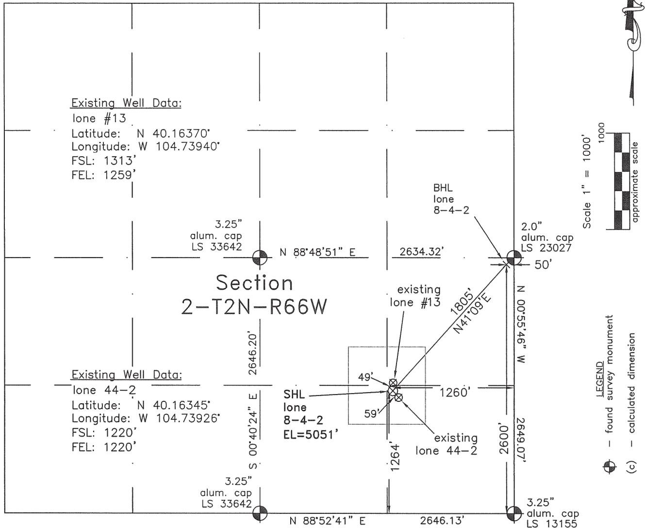
In accordance with a request from Dave Bale of EnCana Oil & Gas (USA) Inc., Frederick Land Surveying, Inc. has determined the location of the **lone 8-4-2** well site to be SHL: 1264' FSL and 1260' FEL, BHL (2600' FSL and 50' FEL) as measured at ninety (90) degrees from the section lines of Section 2, Township 2 North, Range 66 West, 6th Principal Meridian, Weld County, CO.
