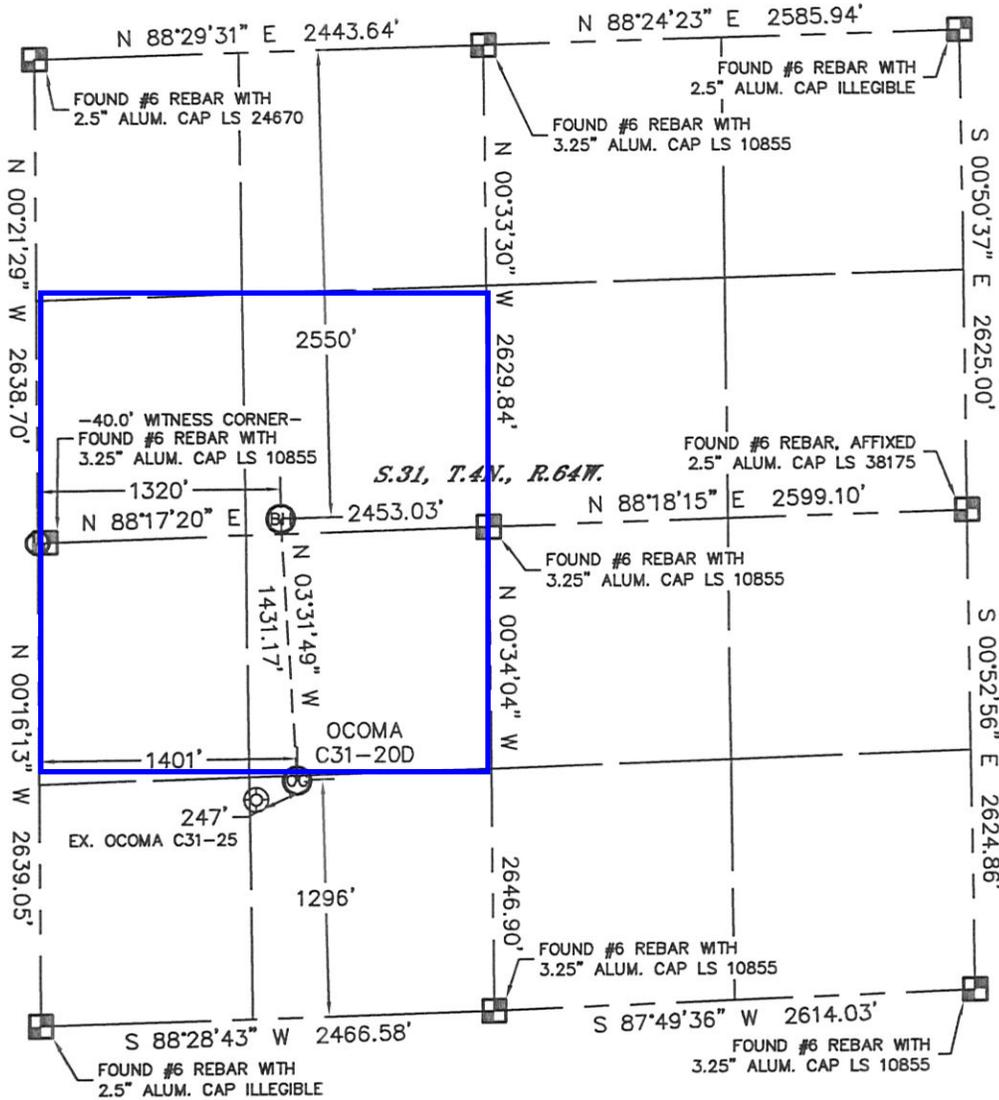
In accordance with a request from Brian DeRose with Noble Energy Inc. Lat40°, Inc. has determined the surface location of the OCOMA C31-20D to be 1296' from the SOUTH line and 1401' from the WEST line and the bottom hole to be 2550' from the NORTH line and 1320' from the WEST line as measured at right angles from the section lines of Section 31, Township 4 North, Range 64 West of the Sixth Principal Meridian, County of Weld, State of Colorado.
