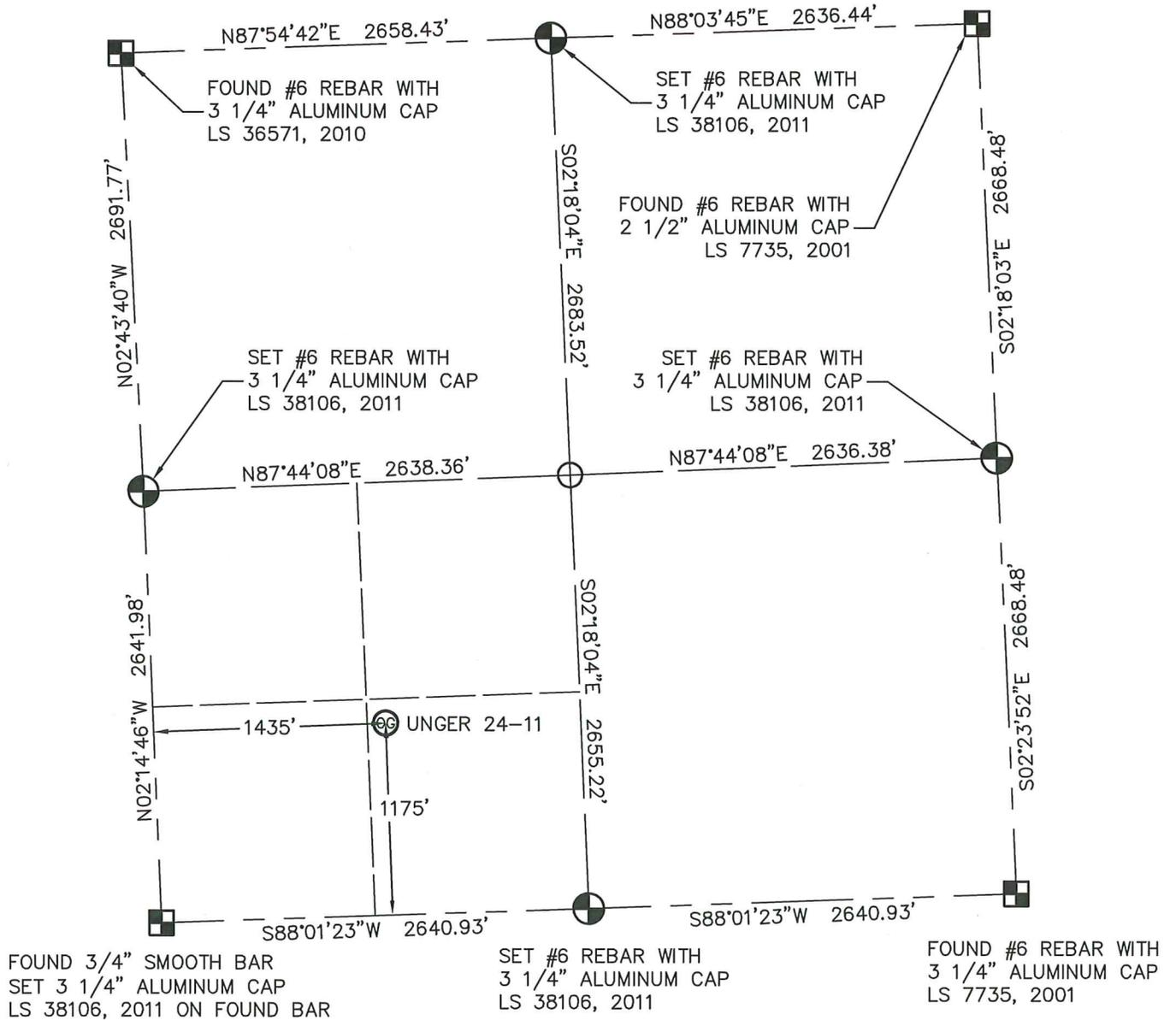
In accordance with a request from DAVID LEDET with NOBLE ENERGY INC. King Surveyors Inc. has determined the surface location of UNGER 24-11 to be 1175' from the SOUTH line and 1435' from the WEST line, as measured at right angles, from the section lines of Section 11, Township 1 North, Range 46 West of the Sixth Principal Meridian, County of Yuma, State of Colorado.
