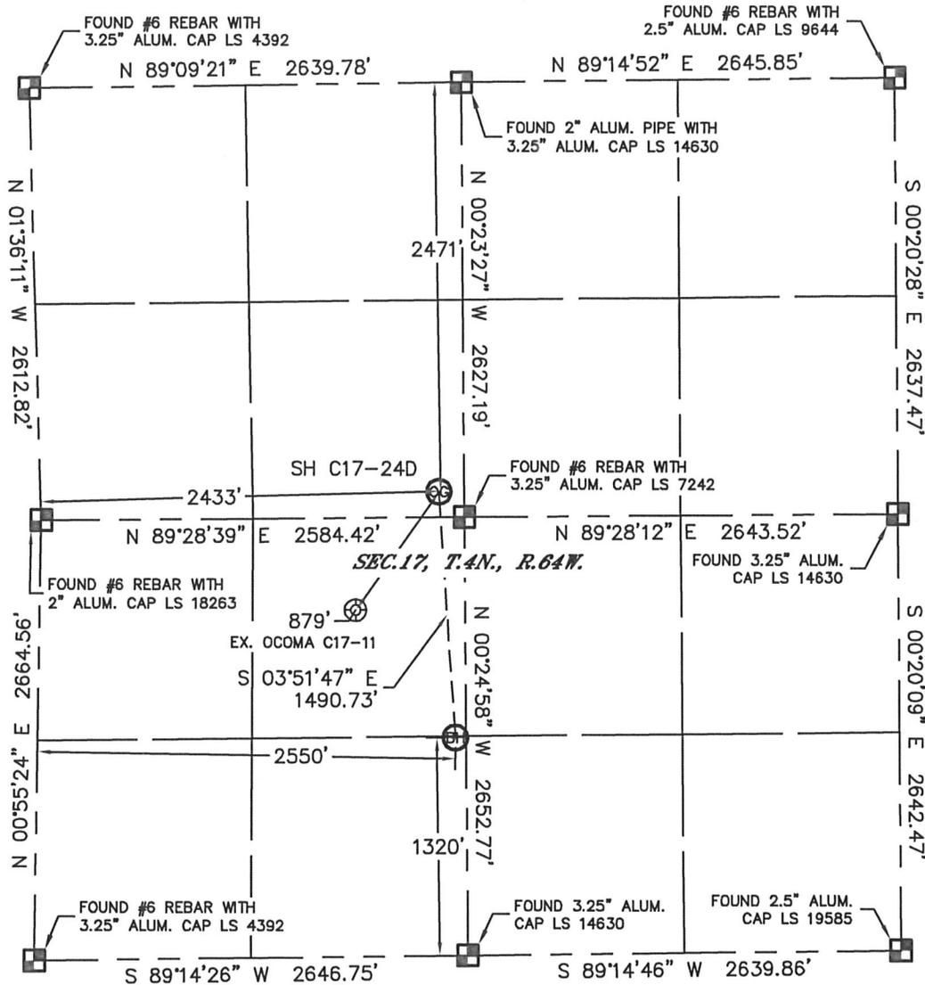
In accordance with a request from Matt Verbit with Noble Energy Inc., Lat40°, Inc. has determined the surface location of the SH C17-24D to be 2471' from the NORTH line and 2433' from the WEST line and the bottom hole to be 1320' from the SOUTH line and 2550' from the WEST line as measured at right angles from the section lines of Section 17, Township 4 North, Range 64 West of the Sixth Principal Meridian, County of Weld, State of Colorado.
