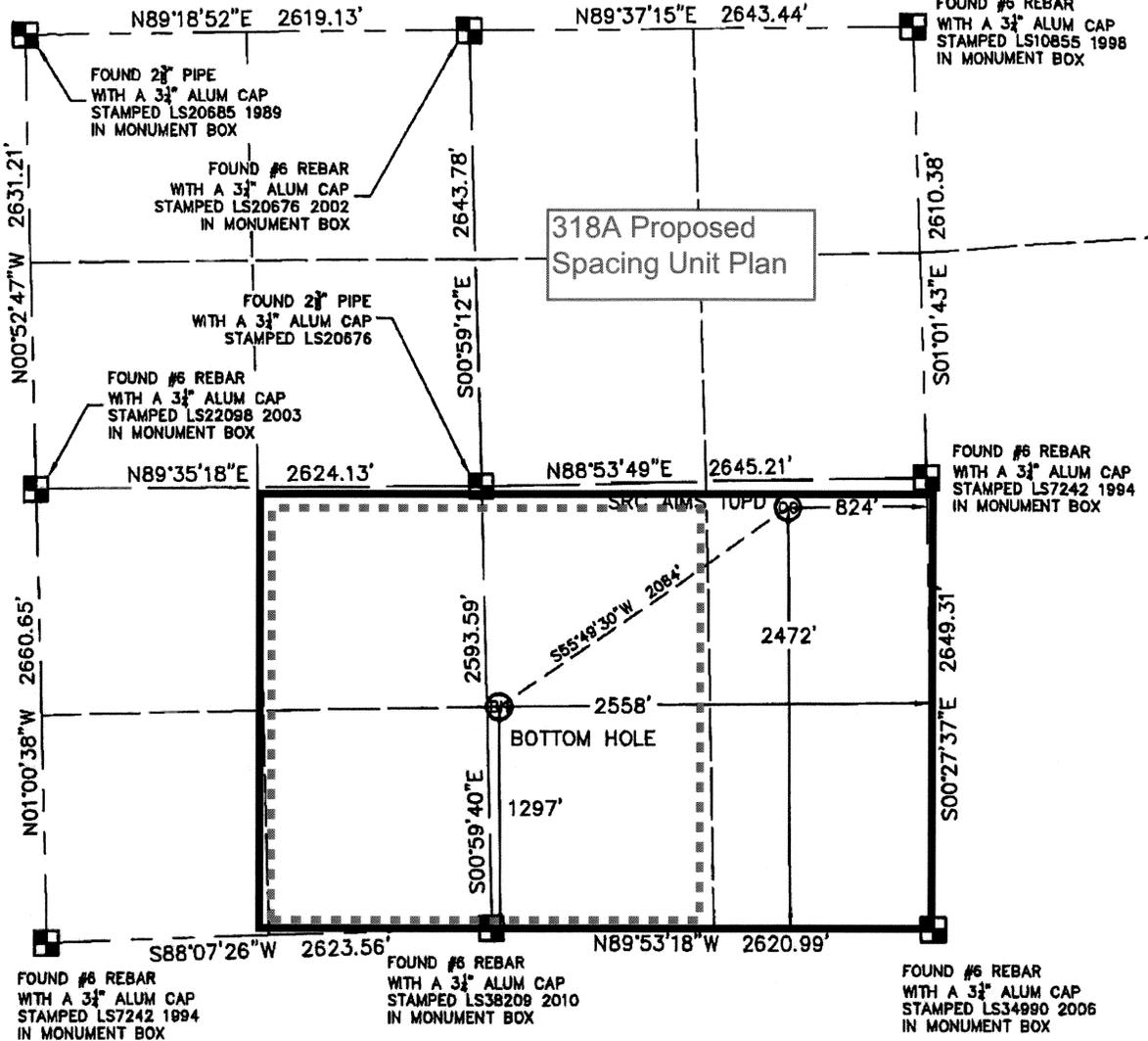
In accordance with a request from CRAIG RASMUSON with SYNERGY RESOURCES CORPORATION King Surveyors Inc. has determined the surface location of SRC AIMS 10PD to be 2472' from the SOUTH line and 824' from the EAST line and the bottom hole to be 1297' from the SOUTH line and 2558' from the EAST line, as measured at right angles, from the section lines of Section 10, Township 5 North, Range 66 West of the Sixth Principal Meridian, County of Weld, State of Colorado.
