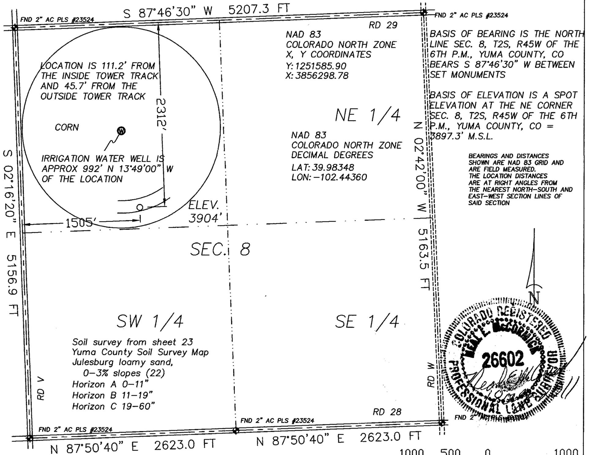
BEARINGS AND DISTANCES SHOWN ARE NAD 83 GRID AND ARE FIELD MEASURED. THE LOCATION DISTANCES ARE AT RIGHT ANGLES FROM THE NEAREST NORTH-SOUTH AND EAST-WEST SECTION LINES OF SAID SECTION
