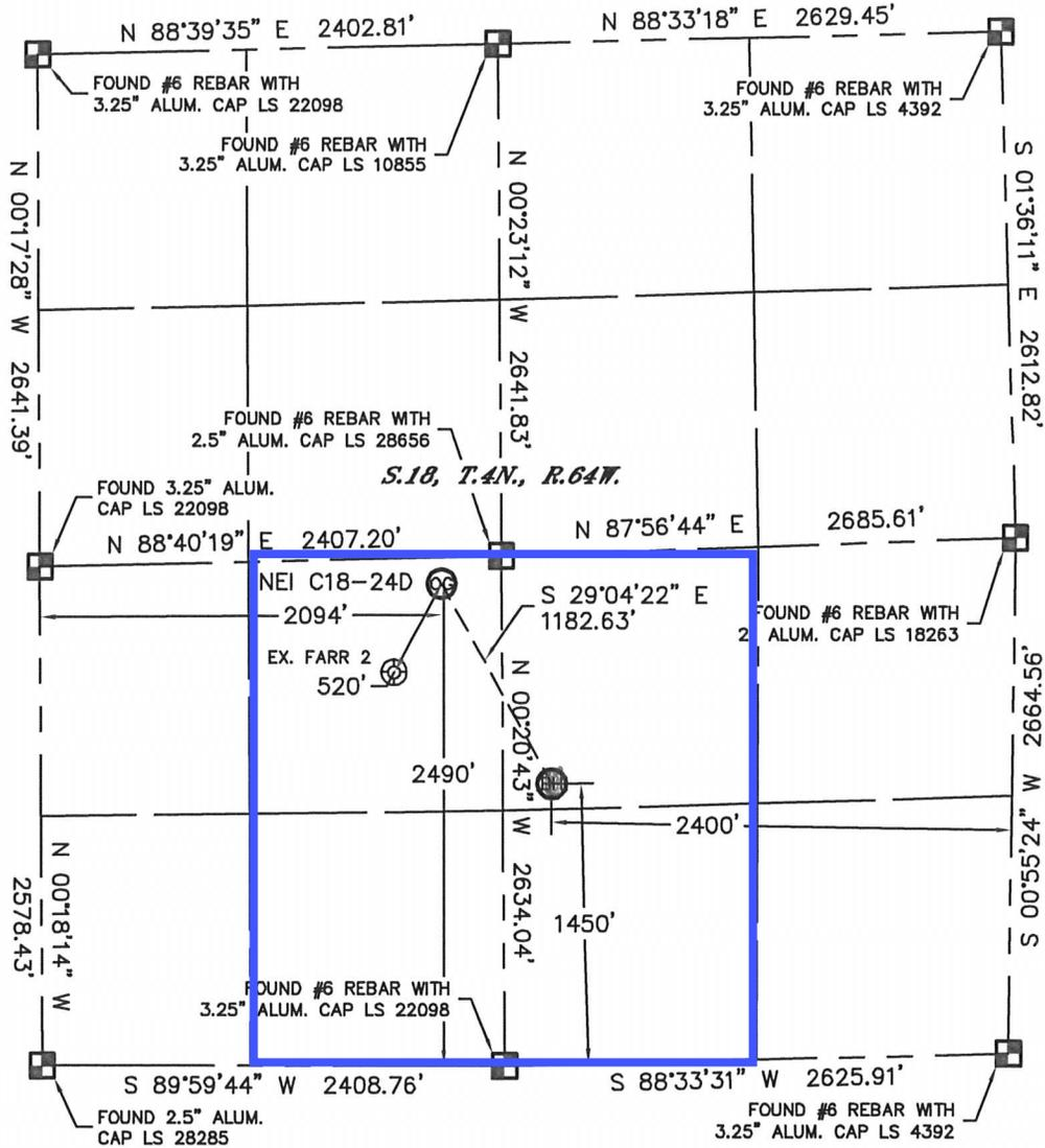
In accordance with a request from Matt Verbit with Noble Energy Inc., Lat40°, Inc. has determined the surface location of the NEI C18-24D to be 2490' from the SOUTH line and 2094' from the WEST line and the bottom hole to be 1450' from the SOUTH line and 2400' from the EAST line as measured at right angles from the section lines of Section 18, Township 4 North, Range 64 West of the Sixth Principal Meridian, County of Weld, State of Colorado.
