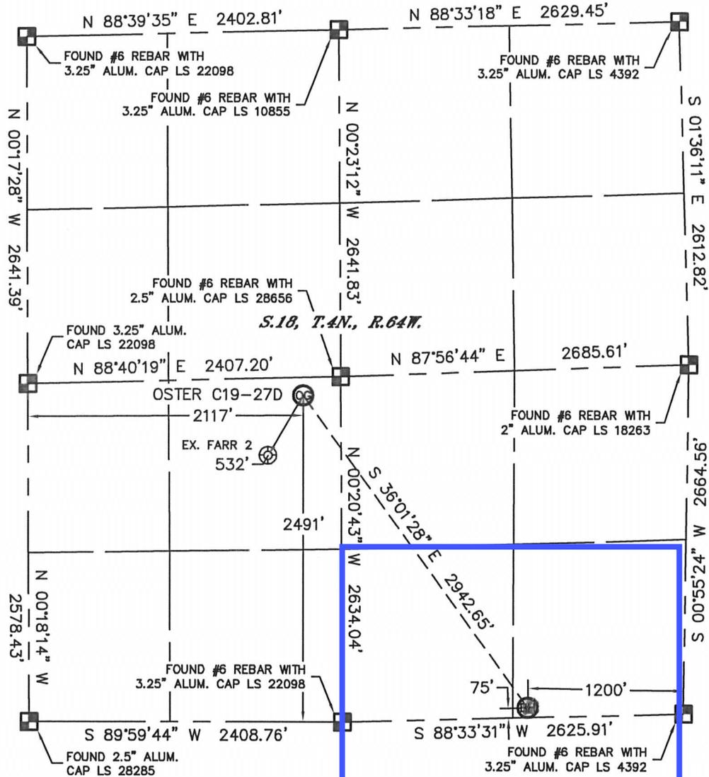
In accordance with a request from Matt Verbit with Noble Energy Inc. Lat40°, Inc. has determined the surface location of the OSTER C19-27D to be 2491' from the SOUTH line and 2117' from the WEST line and the bottom hole to be 75' from the SOUTH line and 1200' from the EAST line as measured at right angles from the section lines of Section 18, Township 4 North, Range 64 West of the Sixth Principal Meridian, County of Weld, State of Colorado.
