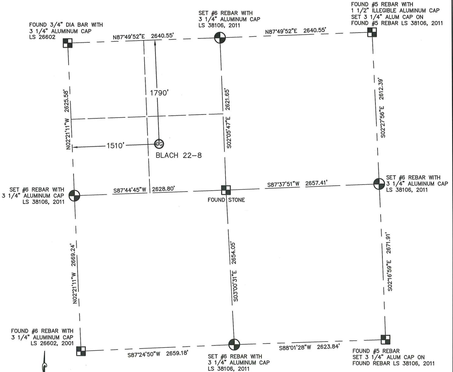
In accordance with a request from DAVID LEDET with NOBLE ENERGY INC. King Surveyors Inc. has determined the surface location of BLACH 22-8 to be 1790' from the NORTH line and 1510' from the WEST line, as measured at right angles, from the section lines of Section 8, Township 1 North, Range 46 West of the Sixth Principal Meridian, County of Yuma, State of Colorado.
