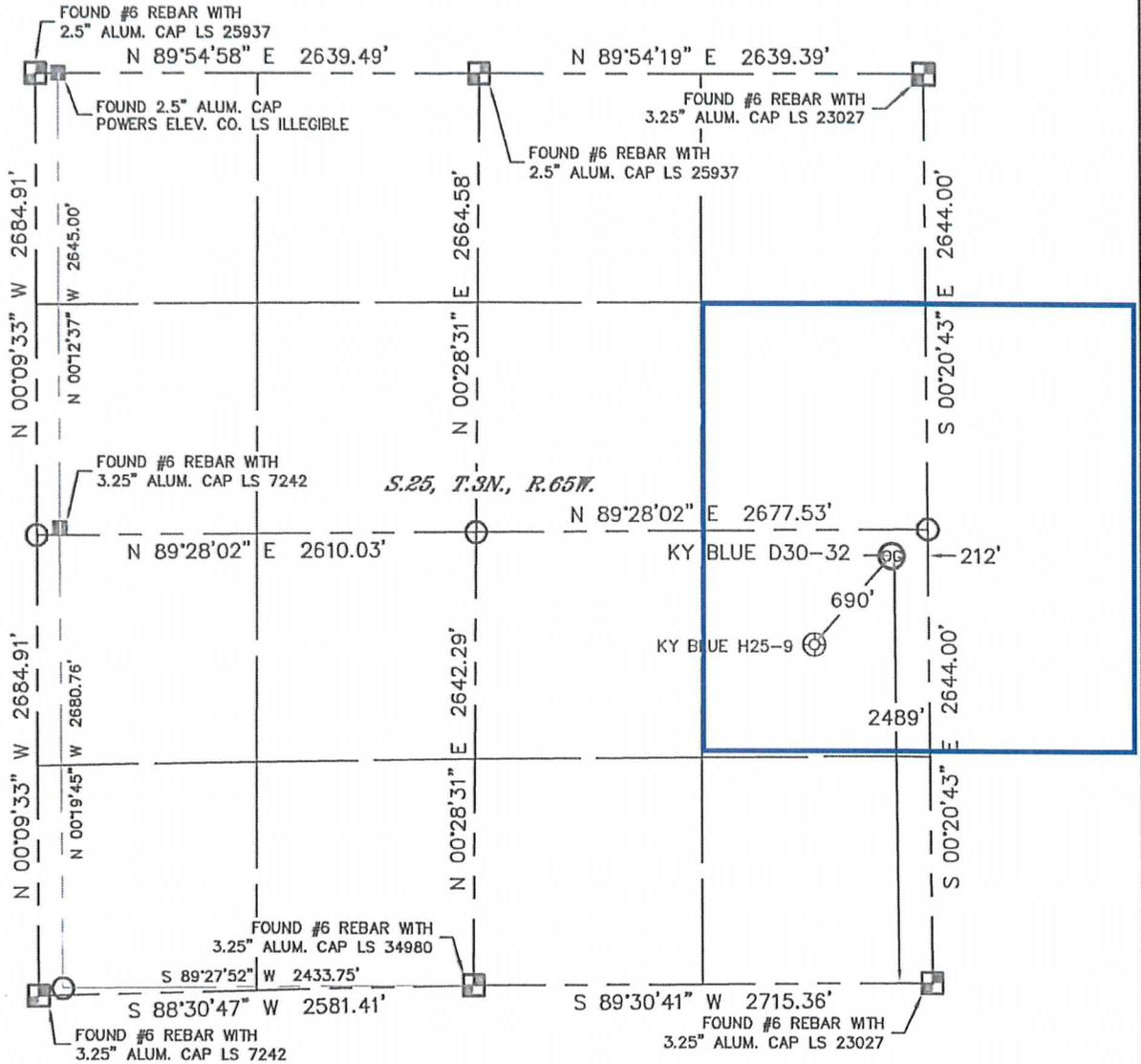
In accordance with a request from Jacob Rice with Noble Energy Inc., Lat40°, Inc. has determined the surface location of the KY BLUE D30-32 to be 2489' from the SOUTH line and 212' from the EAST line as measured at right angles from the section lines of Section 25, Township 3 North, Range 65 West of the Sixth Principal Meridian, County of Weld, State of Colorado.
