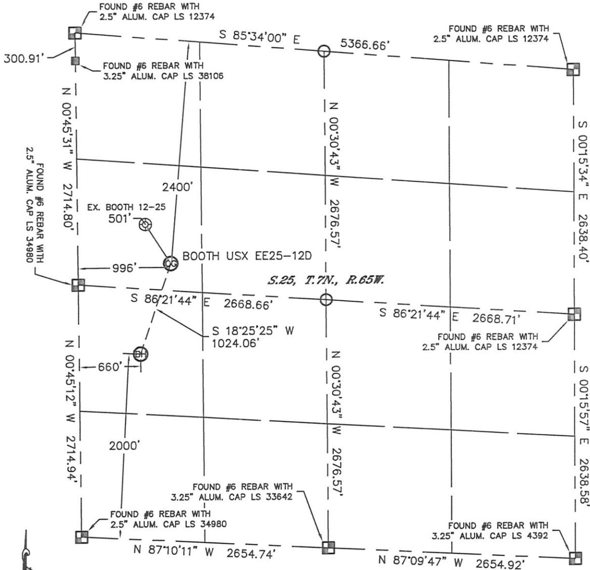
In accordance with a request from Matt Verbit with Noble Energy Inc. Lat40°, Inc. has determined the surface location of the BOOTH USX EE25-12D to be 2400' from the NORTH line and 996' from the WEST line and the bottom hole to be 2000' from the SOUTH line and 660' from the WEST line as measured at right angles from the section lines of Section 25, Township 7 North, Range 65 West of the Sixth Principal Meridian, County of Weld, State of Colorado.
