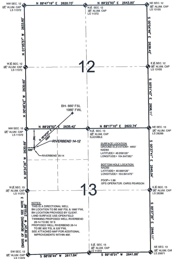
WELL RIVERBEND 14-12 TO BE LOCATED 795' FNL AND 320' FWL, SECTION 13, T1N, R67W OF THE 6th P.M.
