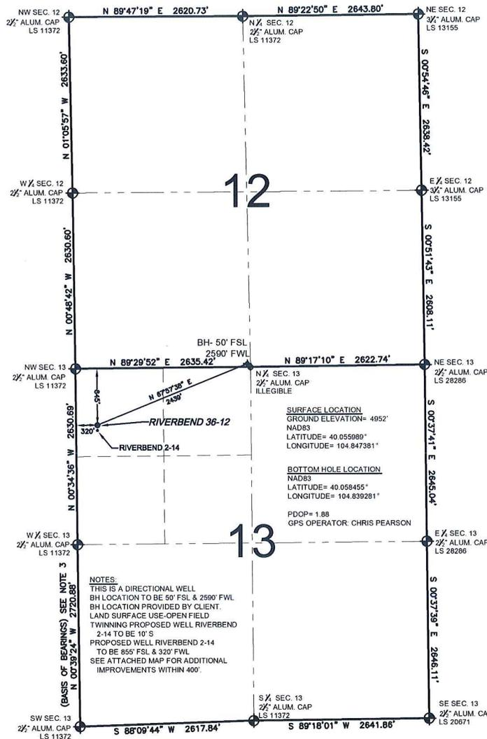
WELL RIVERBEND 36-12 TO BE LOCATED 845' FNL AND 320' FWL, SECTION 13, T1N, R67W OF THE 6th P.M.
