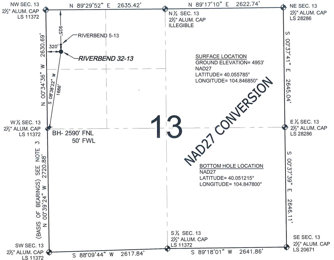
WELL **RIVERBEND 32-13** TO BE LOCATED 925' FNL AND 320' FWL, SECTION 13, T1N, R67W OF THE 6th P.M.
