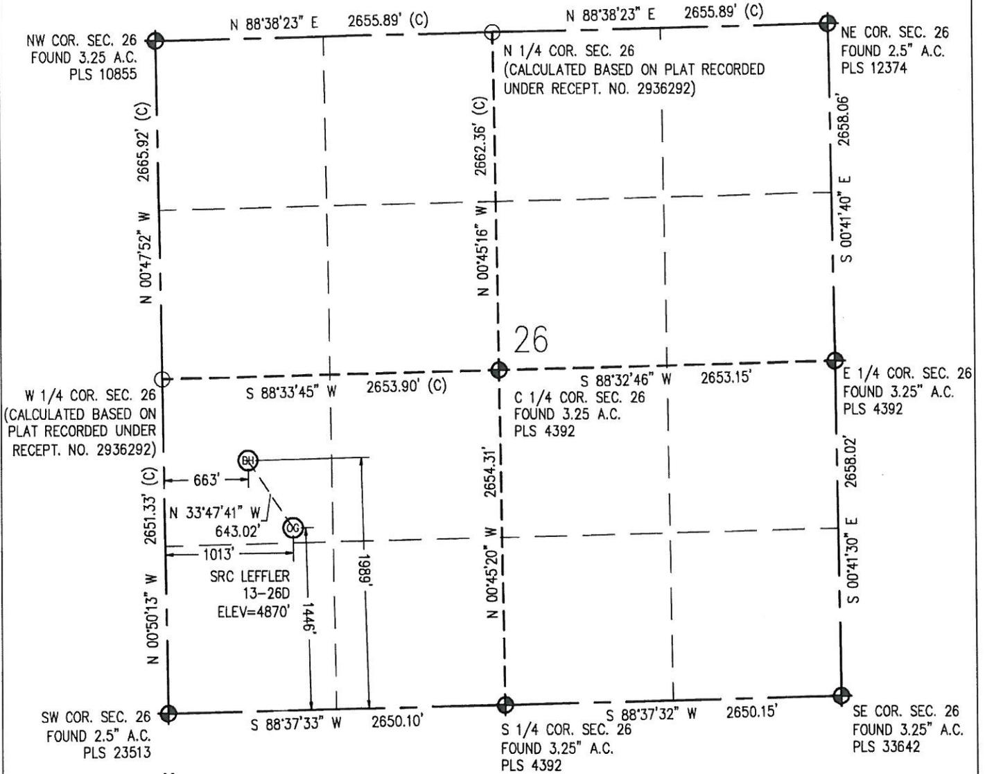
IN ACCORDANCE WITH A REQUEST FROM CRAIG RASMUSON - SYNERGY RESOURCES, BASELINE ENGINEERING CORP. HAS DETERMINED THE LOCATION OF THE SRC LEFFLER 13-26D TO BE 1,446' FSL AND 1,013' FWL AS MEASURED AT NINETY (90) DEGREES FROM THE SECTION LINE OF SECTION 26, TOWNSHIP 7 NORTH, RANGE 66 WEST AND THE BOTTOM HOLE LOCATION TO BE 1,989' FSL AND 663' FWL OF SECTION 26, TOWNSHIP 7 NORTH, RANGE 66 WEST, 6TH PRINCIPAL MERIDIAN, WELD COUNTY, COLORADO.
