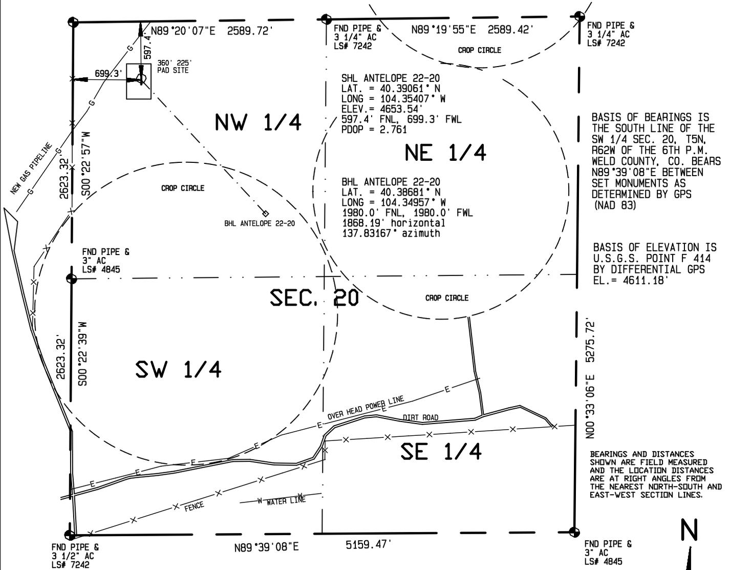
BASIS OF BEARINGS IS THE SOUTH LINE OF THE SW 1/4 SEC. 20, T5N, R62W OF THE 6TH P.M. WELD COUNTY, CO. BEARS N89°39'08\"E BETWEEN SET MONUMENTS AS DETERMINED BY GPS (NAD 83)
