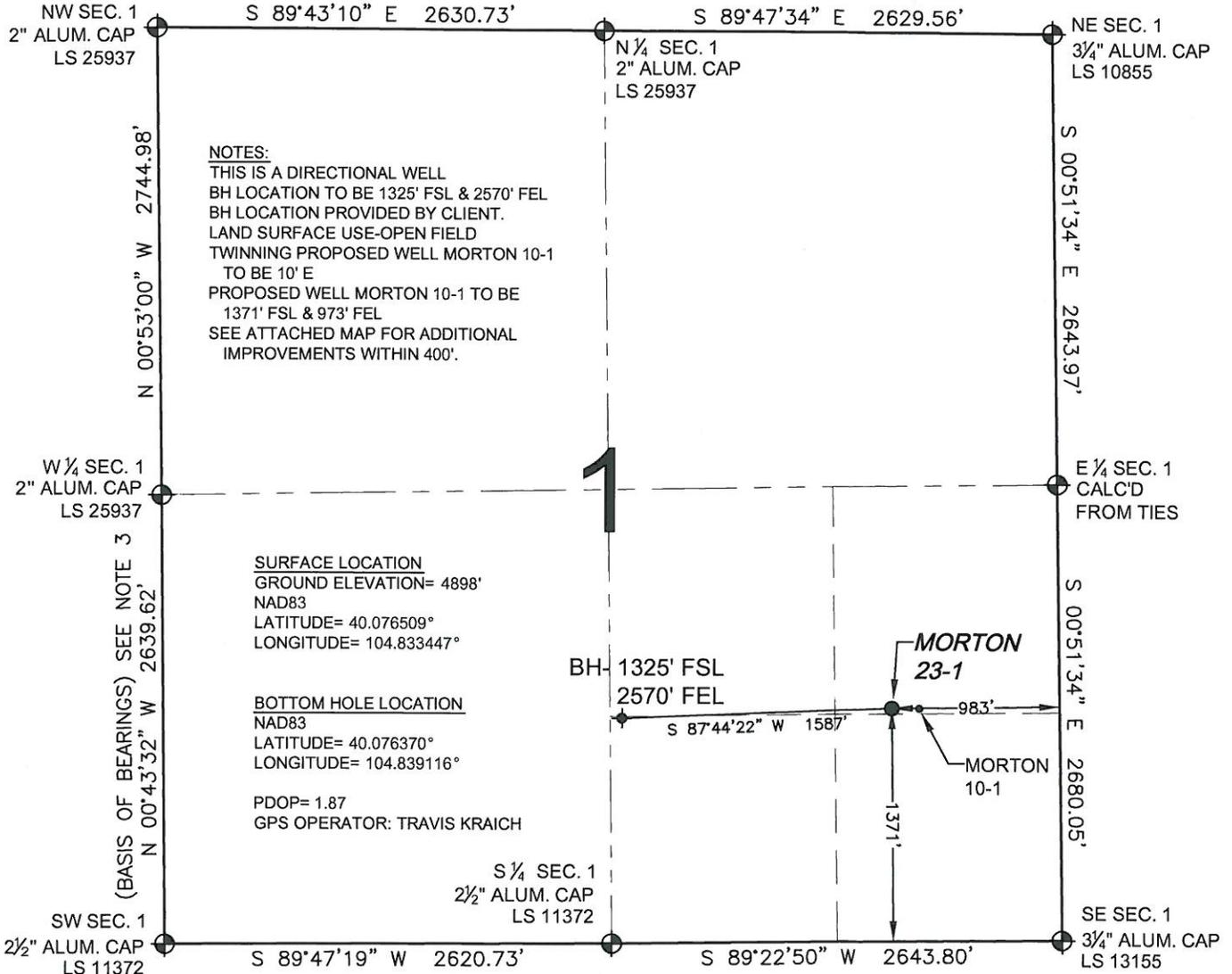
WELL **MORTON 23-1** TO BE LOCATED 1371' FSL AND 983' FEL, SECTION 1, T1N, R67W OF THE 6th P.M.
