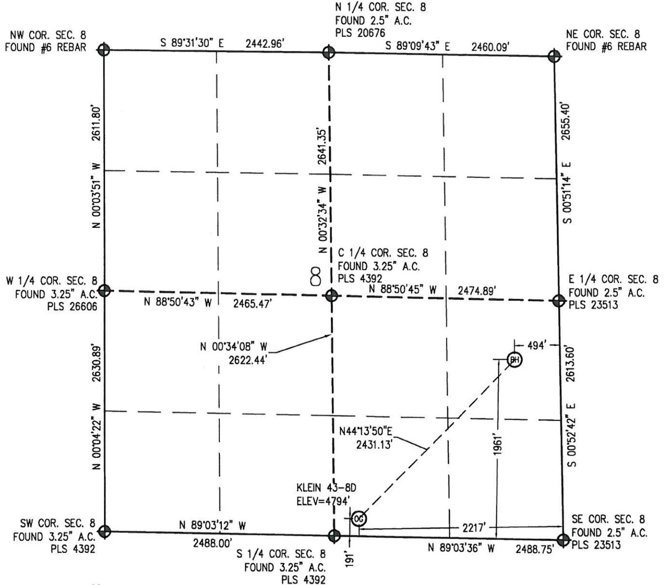
IN ACCORDANCE WITH A REQUEST FROM CRAIG RASMUSON - SYNERGY RESOURCES, BASELINE ENGINEERING CORP. HAS DETERMINED THE LOCATION OF THE KLEIN 43-8D TO BE 191' FSL AND 2,217' FEL, AS MEASURED AT NINETY (90) DEGREES FROM THE SECTION LINE OF SECTION 8, TOWNSHIP 4 NORTH, RANGE 67 WEST AND THE BOTTOM HOLE LOCATION TO BE 1,961' FSL AND 494' FEL OF SECTION 8, TOWNSHIP 4 NORTH, RANGE 67 WEST, 6TH PRINCIPAL MERIDIAN, WELD COUNTY, COLORADO.
