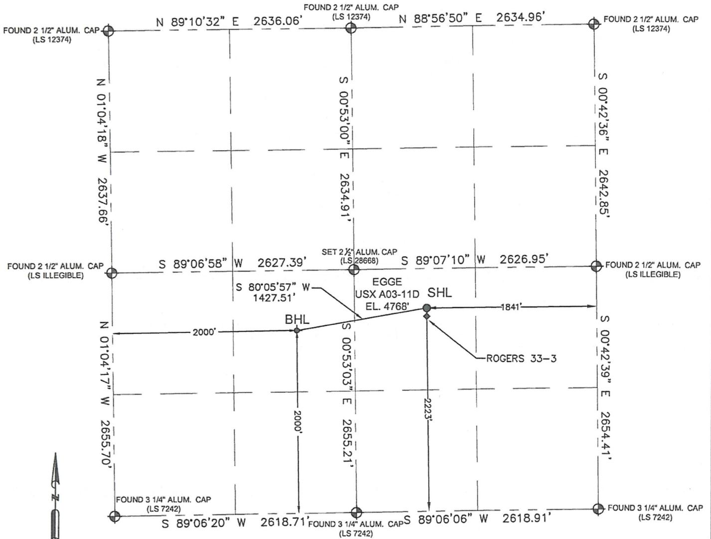
In accordance with a request from CJ Pietri with Noble Energy Inc. Petroleum Field Services, LLC has determined the surface location of the EGGE USX A03-11D to be 2223' from the SOUTH line and 1841' from the EAST line and the bottom hole to be 2000' from the SOUTH line and 2000' from the WEST line as measured at right angles from the section line of Section 3, Township 6 North, Range 64 West of the Sixth Principal Meridian, County of WELD, State of Colorado.
