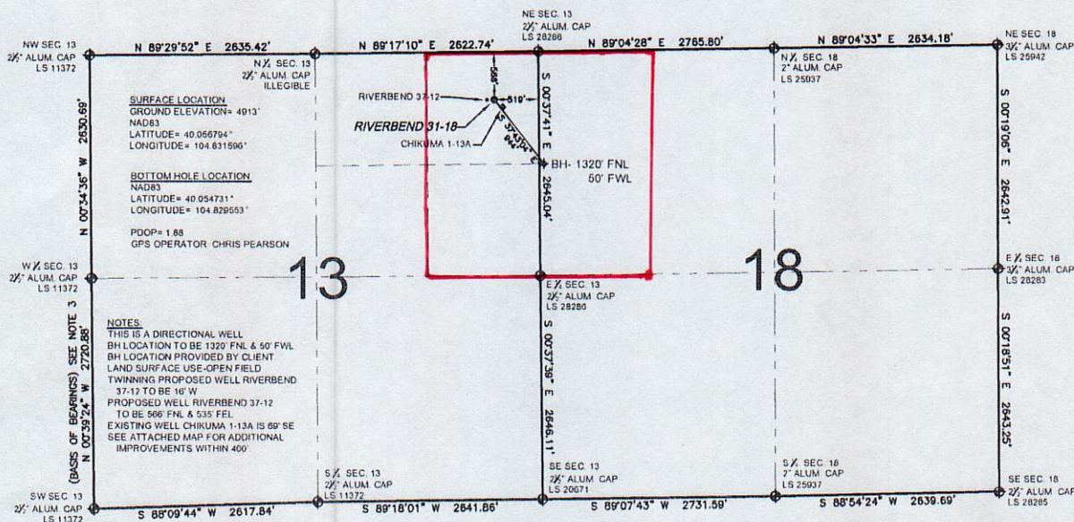
WELL **RIVERBEND 31-18** TO BE LOCATED 566' FNL AND 519' FEL, SECTION 13, T1N, R67W OF THE 6th P.M.
