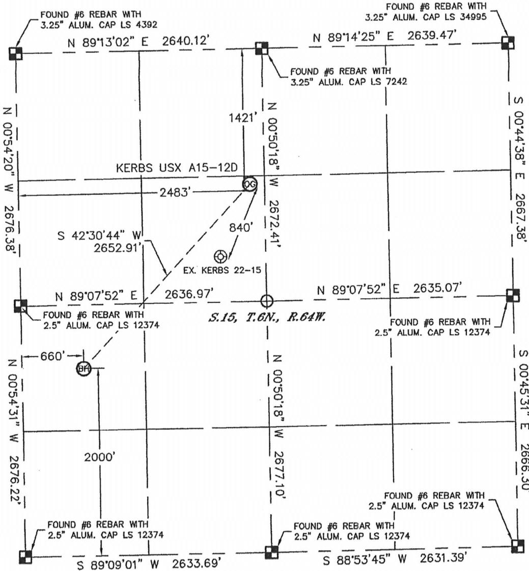
In accordance with a request from Matt Campbell with Noble Energy Inc. Lat40°, Inc. has determined the surface location of the KERBS USX A15-12D to be 1421' from the NORTH line and 2483' from the WEST line and the bottom hole to be 2000' from the SOUTH line and 660' from the WEST line as measured at right angles from the section lines of Section 15, Township 6 North, Range 64 West of the Sixth Principal Meridian, County of Weld, State of Colorado.
