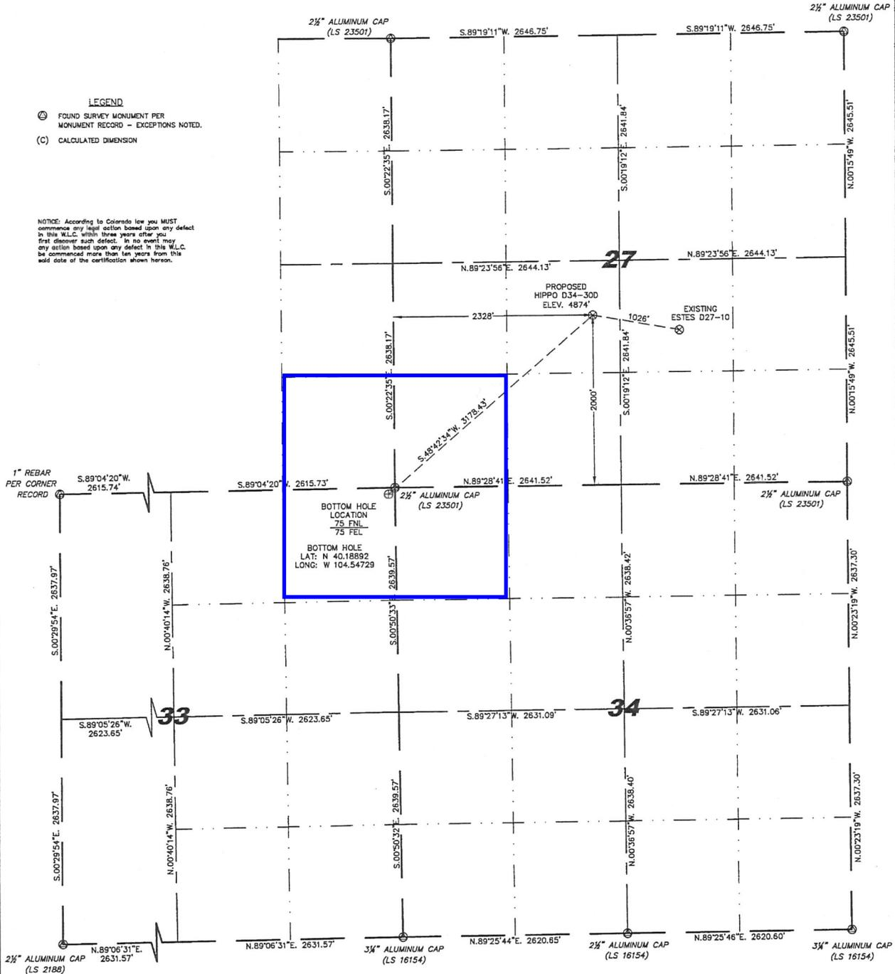
IN ACCORDANCE WITH A REQUEST FROM BRIAN D'ROSE - NOBLE ENERGY INC. STELL SURVEYING SERVICES, LLC HAS DETERMINED THE LOCATION OF THE HIPPO D34-300 WELL TO BE 2000' FSL, 2338' FWL AS MEASURED AT NINETY (90) DEGREES FROM THE SECTION LINES, SECTION 27, TOWNSHIP 3 NORTH, RANGE 64 WEST, 6TH PRINCIPLE MERIDIAN, WELD COUNTY, COLORADO.
