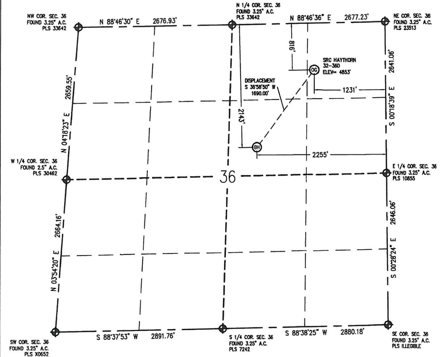
IN ACCORDANCE WITH A REQUEST FROM CRAIG RASMUSON - SYNERGY RESOURCES CORP., BASELINE ENGINEERING CORP. HAS DETERMINED THE LOCATION OF THE SRC HAYTHORN 32-36D TO BE 816' NML AND 1231' FEL, AS MEASURED AT NINETY (90) DEGREES FROM THE SECTION LINE OF SECTION 36, TOWNSHIP 7 NORTH, RANGE 66 WEST AND THE BOTTOM HOLE LOCATION TO BE 2143' NML AND 2255' FEL OF SECTION 36, TOWNSHIP 7 NORTH, RANGE 66 WEST, 6TH PRINCIPAL MERIDIAN, WELD COUNTY, COLORADO.
