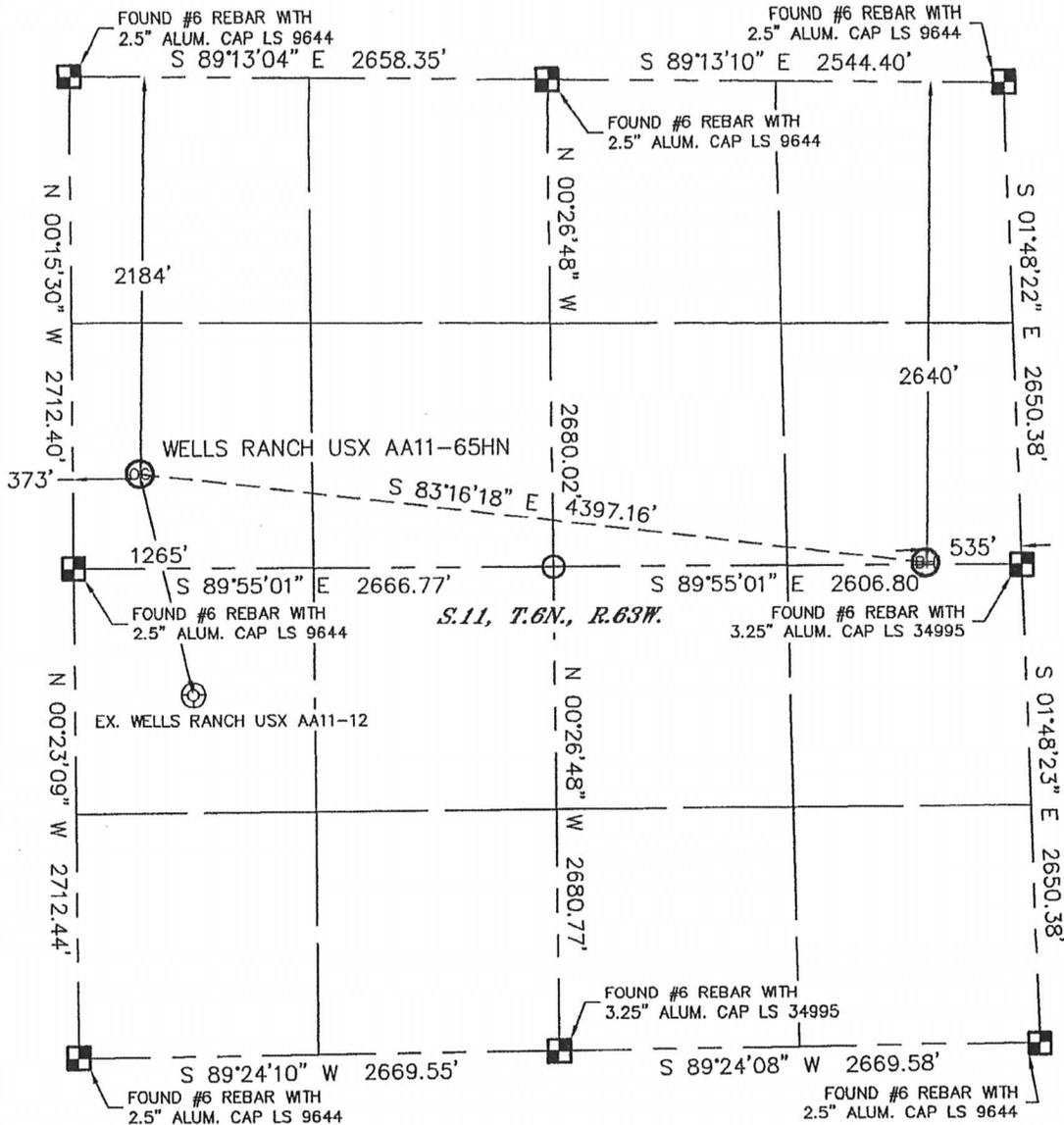
In accordance with a request from Sean Casper with Noble Energy Inc., Lat40°, Inc. has determined the surface location of the WELLS RANCH USX AA11-65HN to be 2184' from the NORTH line and 373' from the WEST line and the bottom hole to be 2640' from the NORTH line and 535' from the EAST line as measured at right angles from the section lines of Section 11, Township 6 North, Range 63 West of the Sixth Principal Meridian, County of Weld, State of Colorado.
