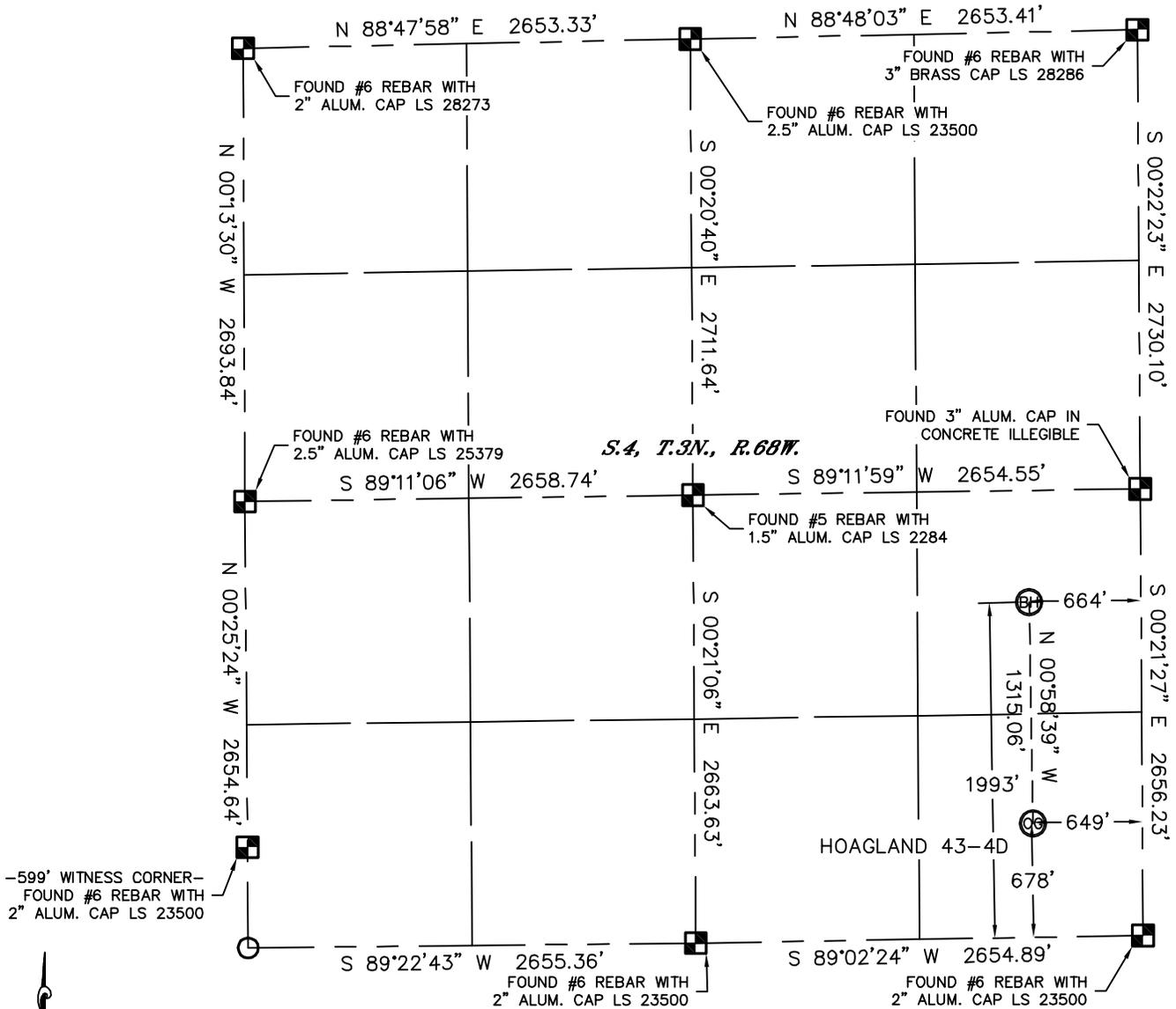
In accordance with a request from Nick Granruth with APOLLO OPERATING, LLC Lat40°, Inc. has determined the surface location of the HOAGLAND 43-4D to be 678' from the SOUTH line and 649' from the EAST line and the bottom hole to be 1993' from the SOUTH line and 664' from the EAST line as measured at right angles from the section lines of Section 4, Township 3 North, Range 68 West of the Sixth Principal Meridian, County of Weld, State of Colorado.
